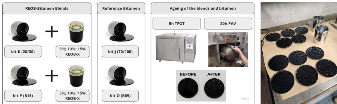
**Figure 3.4: (left) REOB-bitumen blends, the reference bitumen & ageing procedure and (right) TFOT+20hPAV aged bit-K+10% and bit-P+10% blends**
