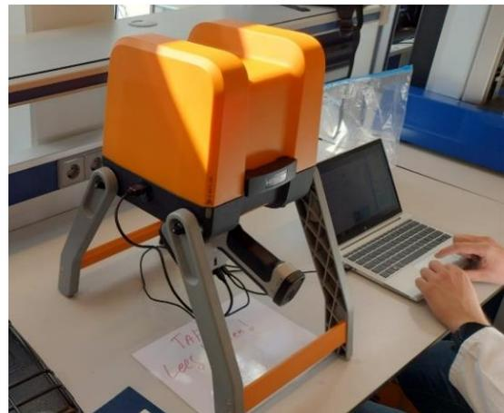
**Figure 4.1: Handheld XRF scanner as benchtop**
