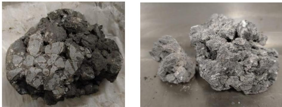
**Figure 7.32: “ravelled” asphalt mixtures with bit-J after dry (left) and Freeze-Thaw conditioning (right) Cantabro Abrasion test (more damage is visible after conditioning)**
