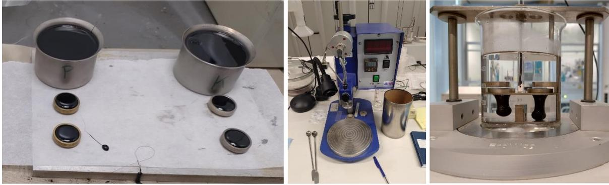
**Figure 3.5: (left) PEN and R&B test samples, (middle) PEN test apparatus and (right) the Ring&Ball test**
