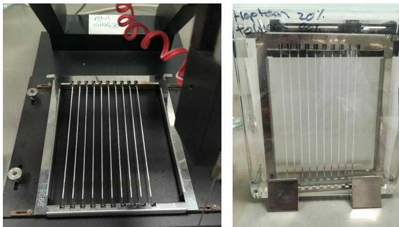
**Figure 4.34: (left) metal frame with quartz rods, in which the bituminous samples can be injected and (right) the metal frame placed in a heptane-toluene (20/80) solution**
