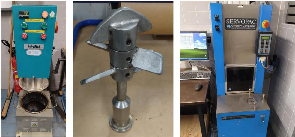
**Figure 7.21: (Left) mixture blender with heated pan; (middle) spindle for the mixture which can also rotate its axis and (right) the gyrator mixture compactor**
