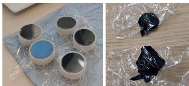
**Figure 4.2: (left) REOB samples for XRF scanning; (right) cooled bitumen samples wrapped in plastic foil**
