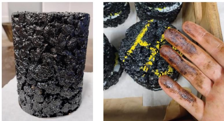
**Figure 7.22: (Left) One gyrator sample of ZOAB+ and (right) after making the samples and before storage at ~15 [°C], the samples were cut. The hand shows that an oil (or REOB) seems to still exudate from the binder, significantly more in the case of bit-K+15% than for bit-J.**
