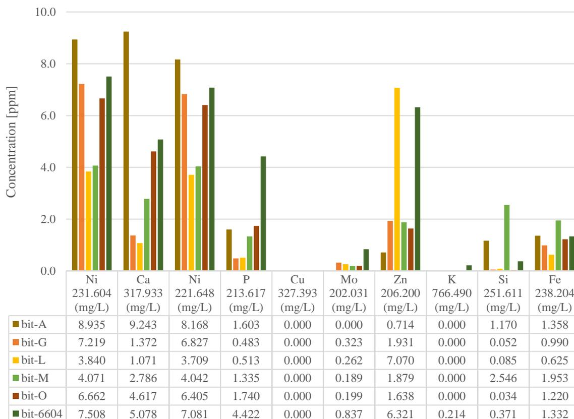
**Figure 4.5: Trace elements found with ICP-AES for unmodified bitumen**
