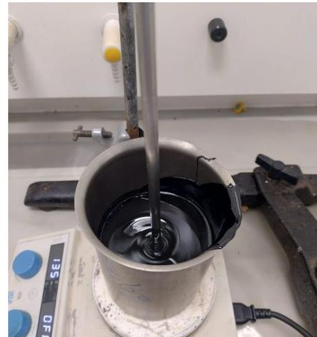
**Figure 3.3: Blending of bitumen and REOB with a low-shear device (200-300 rpm) and keeping the blend warm at 135 [°C]**
