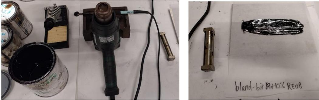
**Figure 7.3: (left) thermal scoop, heat gun and metal rod and (right) a spread-out bitumen thin film on silicon paper**
