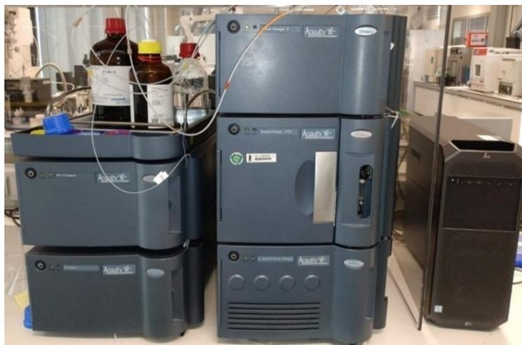
**Figure 4.51: Waters Acquity GPC setup to measure intensities of molecules at specific elution volumes/retention times**
