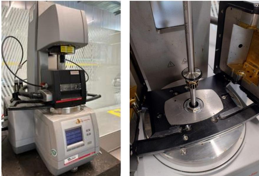
**Figure 5.1: (left) Modular Compact Rheometer MCR 502, Anton Paar and (right) bitumen sample ready for the excess bitumen to be cut and then be tested**
