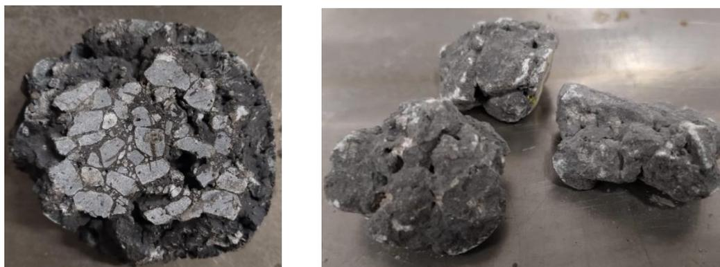
**Figure 7.33: “ravelled” asphalt mixtures with bit-K+15% after dry (left) and Freeze-Thaw conditioning (right) Cantabro Abrasion test (significantly more damage is visible after conditioning)**
