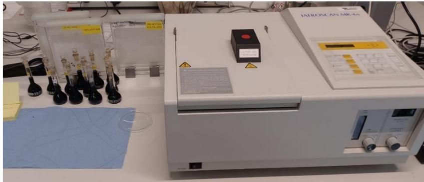
**Figure 4.33: Iatroskan for performing the SARA analysis using different solutions to dissolve the bitumen**
