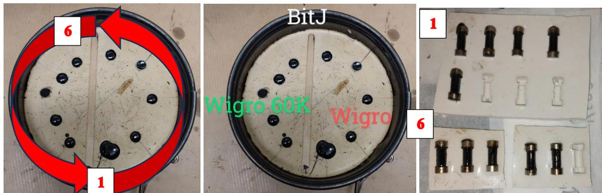
**Figure 7.14: Mastic columns poured in mould with bit-J started at position 1 with Wigro filler, continuing counter-clockwise and starting with Wigro 60K at position 6 (left and middle pictures) and samples placed in another mould ready for testing (right picture)**
