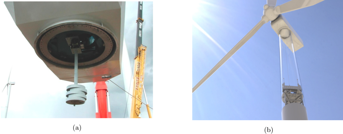
Figure 3: Tuned mass dampers used in the wind turbine industry (a) TMD mounted below the nacelle [22] [Source: ESM GMBh] (b) Artistic impression of TMD mounted in the tower of the turbine [23] [Source: Xi Engineering consultants]
