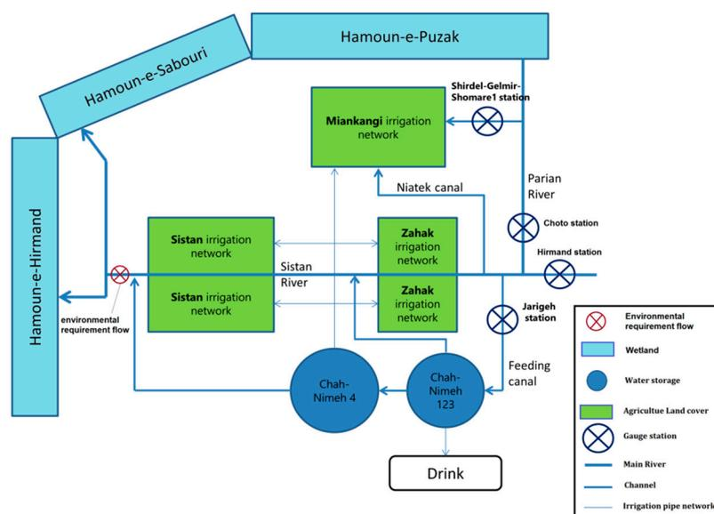
**Figure 2.** Schematic model of the water system in Sistan region, Iran.
