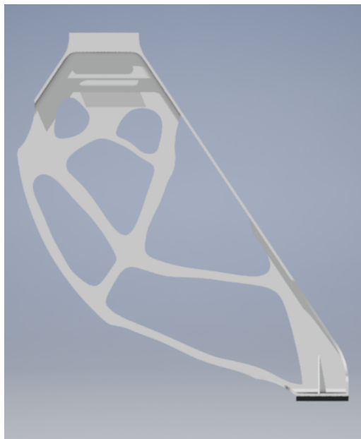
Figure 8.23: Optimized landing gear with rubber feet
