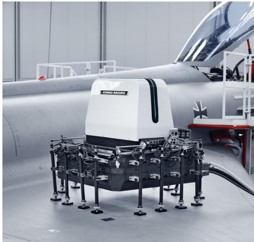
Figure 5.2: ULTRASONIC mobileBLOCK attached to an aircraft fuselage 1
