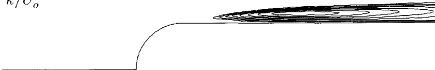
Figure 5.20: T3L6 flow: Computed stream-lines and contours of turbulence kinetic energy k/U_o^2 (contour interval by 0.05) obtained with SMC. Separation point is at x_S/R = 0.9296 and reattachment point is x_R/R = 3.438 . Inlet: U_o = 10m/s , u/U_o = 0.0286 and L_\epsilon = 0.0125m .
