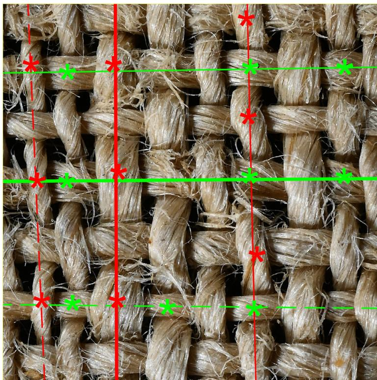
**Fig. 3.** Yarns in warp (red) and weft (green) selected as representative of the Small (S), Medium (M) and Large (L) width subsets within the 1cm<sup>2</sup> observation area, and the observation points.
