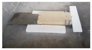
(b) Sandstone sample in place and clamped (T.Rutten [11])
