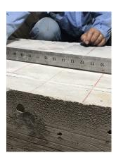
Figure A.2: Visible uneven surface of block
