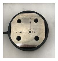
Figure 3.3: Load sensor type: KD43050K
