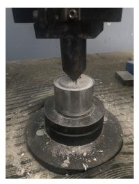
(a) Configuration concrete indentation test
