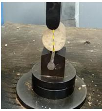
(a) Visible central splitting of sample 4 due to tensile stresses
