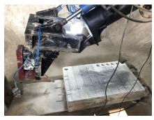
(a) Concrete sample in place on transition piece
