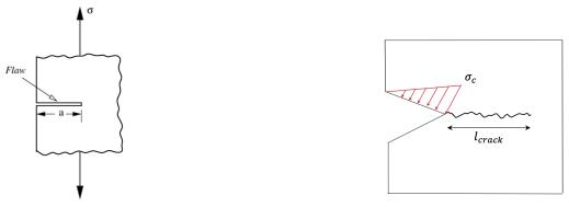
(a) Crack loading according to Griffith [16]
