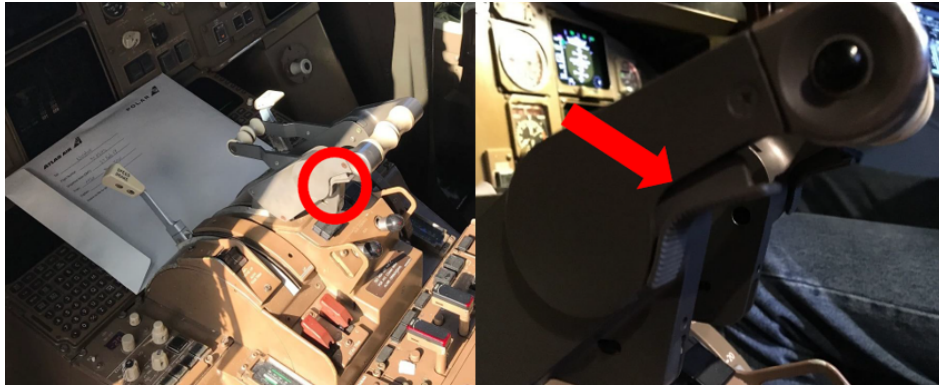
Figure 4-7: Location of GA switches, the red circle indicates the left GA switch. Photo taken of exemplar B-767 by NTSB investigators on February 27, 2019 [14]
