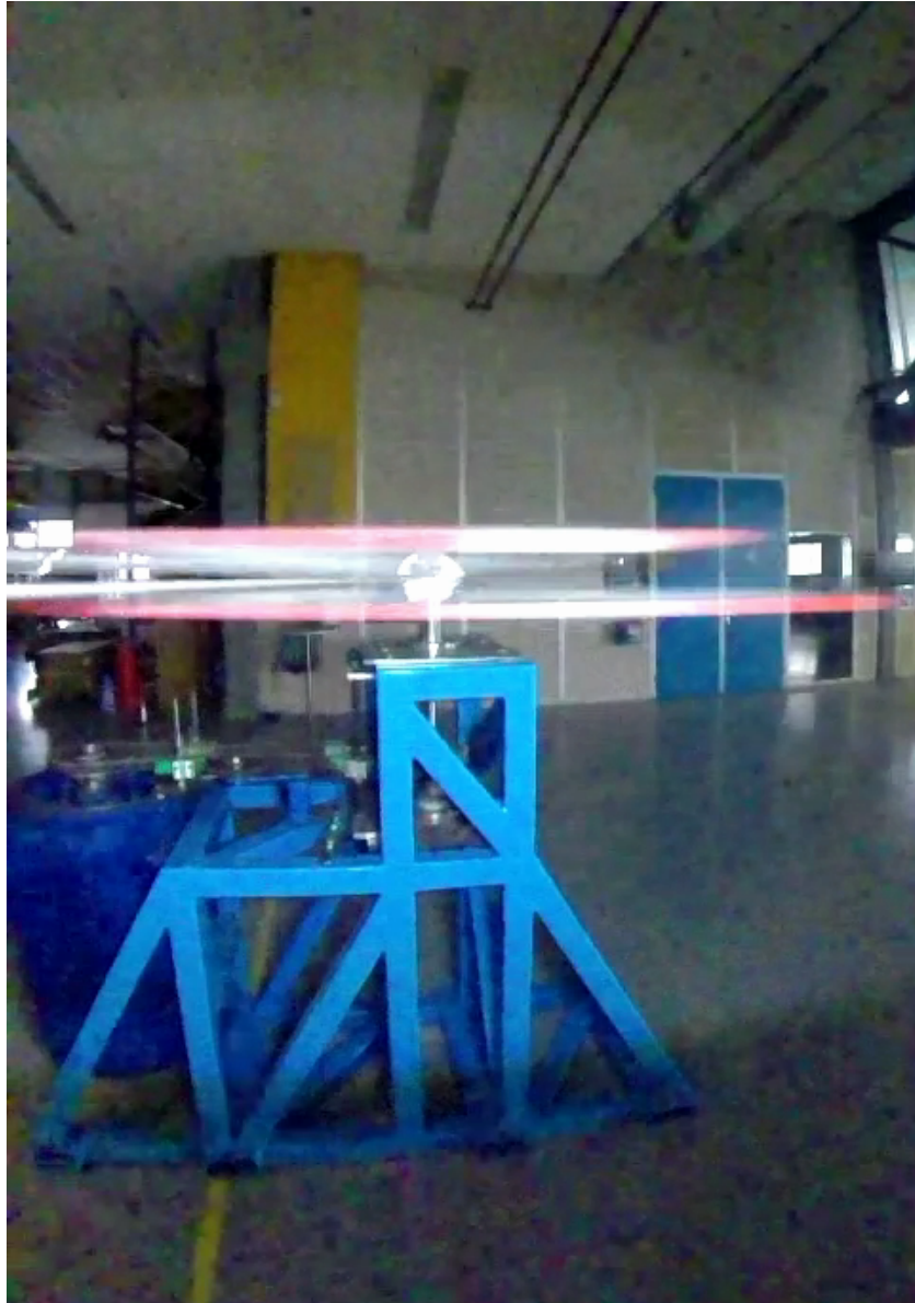
Figure 5.10: Blade deflection at 0^\circ and at 7^\circ collective
