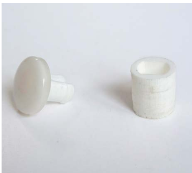
The first test print of the button snap fit
