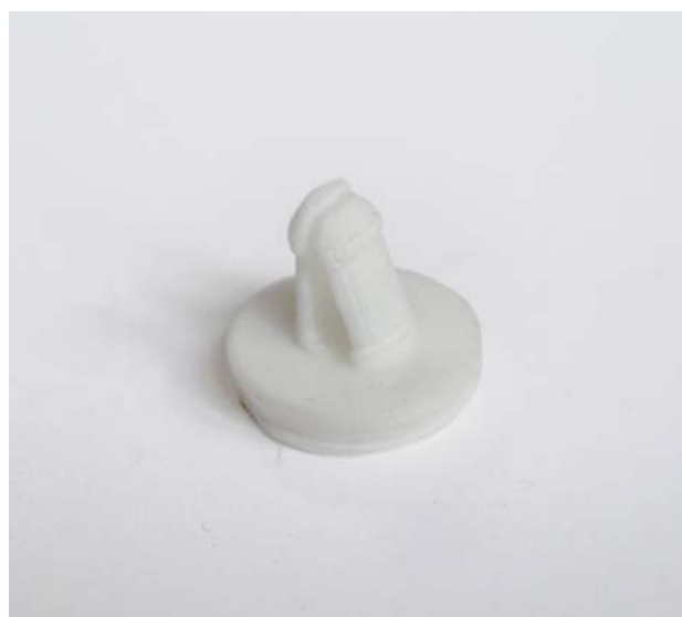
Early designs tend to break at their snap base
