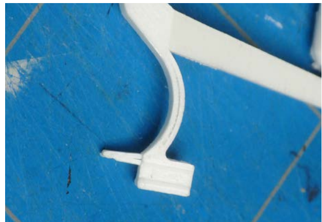
The result of test 3: another damaged spring and displaced valve
