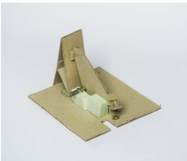
A quick model to test the feel of a magnet system
