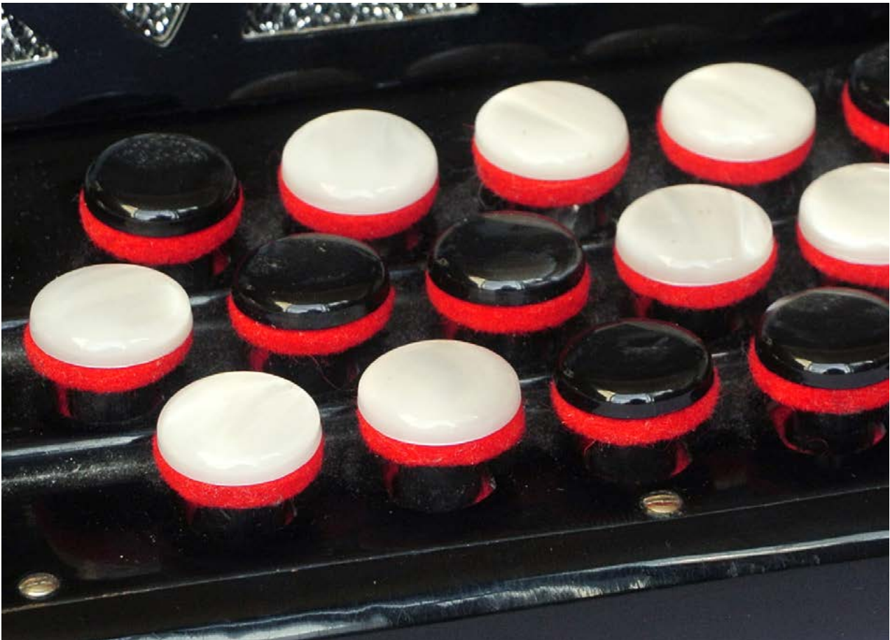
The buttons on a conventional instrument, with felt glued onto the bottom
