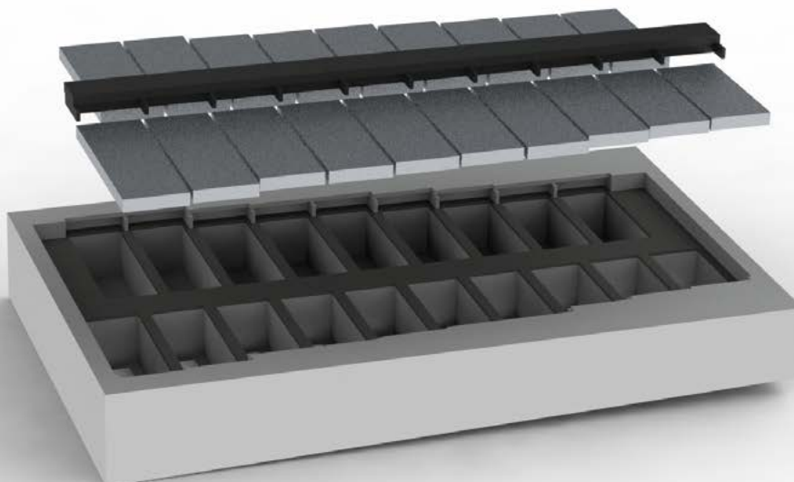
Early impression of the reed block with a single mounting bar in the middle. This is the same basic principle as in the final design, although the mounting bar has been split up into pieces and the chamber dimensions have changed.
