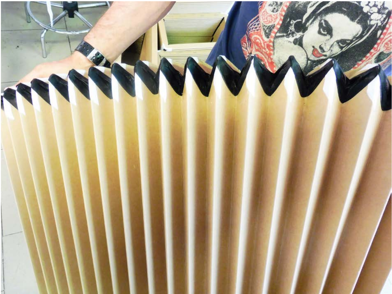
A bellows during production. The cardboard base has been established, the corners are covered by leather. Applying fabric is the next step.
