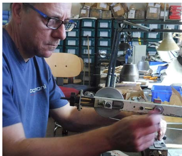
A reed is pretuned after assembly. After accordion construction, all reeds are tuned once more, this time more precise.
