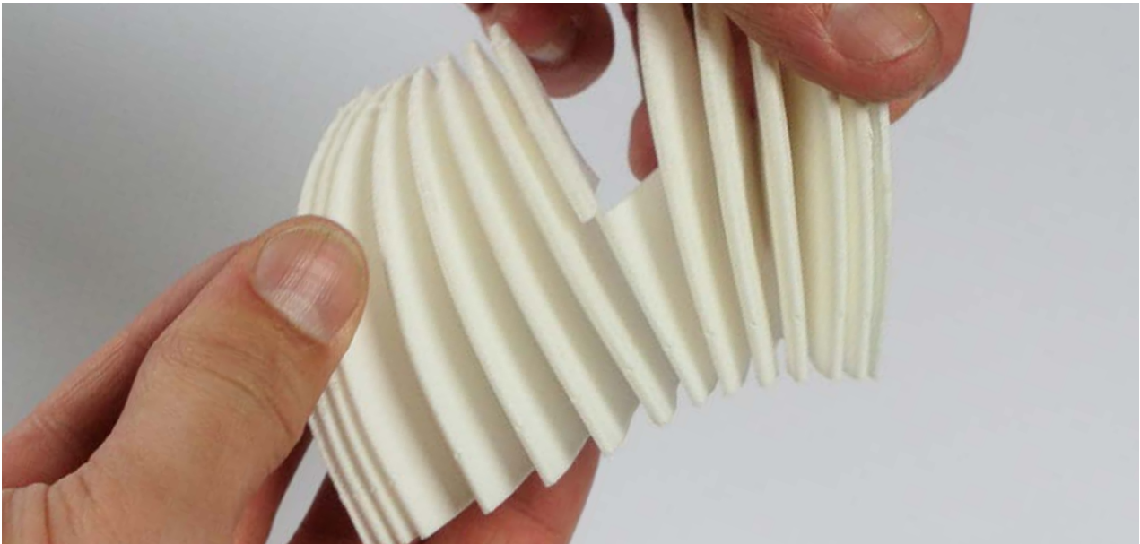
Prints tend to break along the material layers. The bellow planes are oriented in two different directions, and the third direction is used for bellow movement. This makes print layer orientation a problem.
