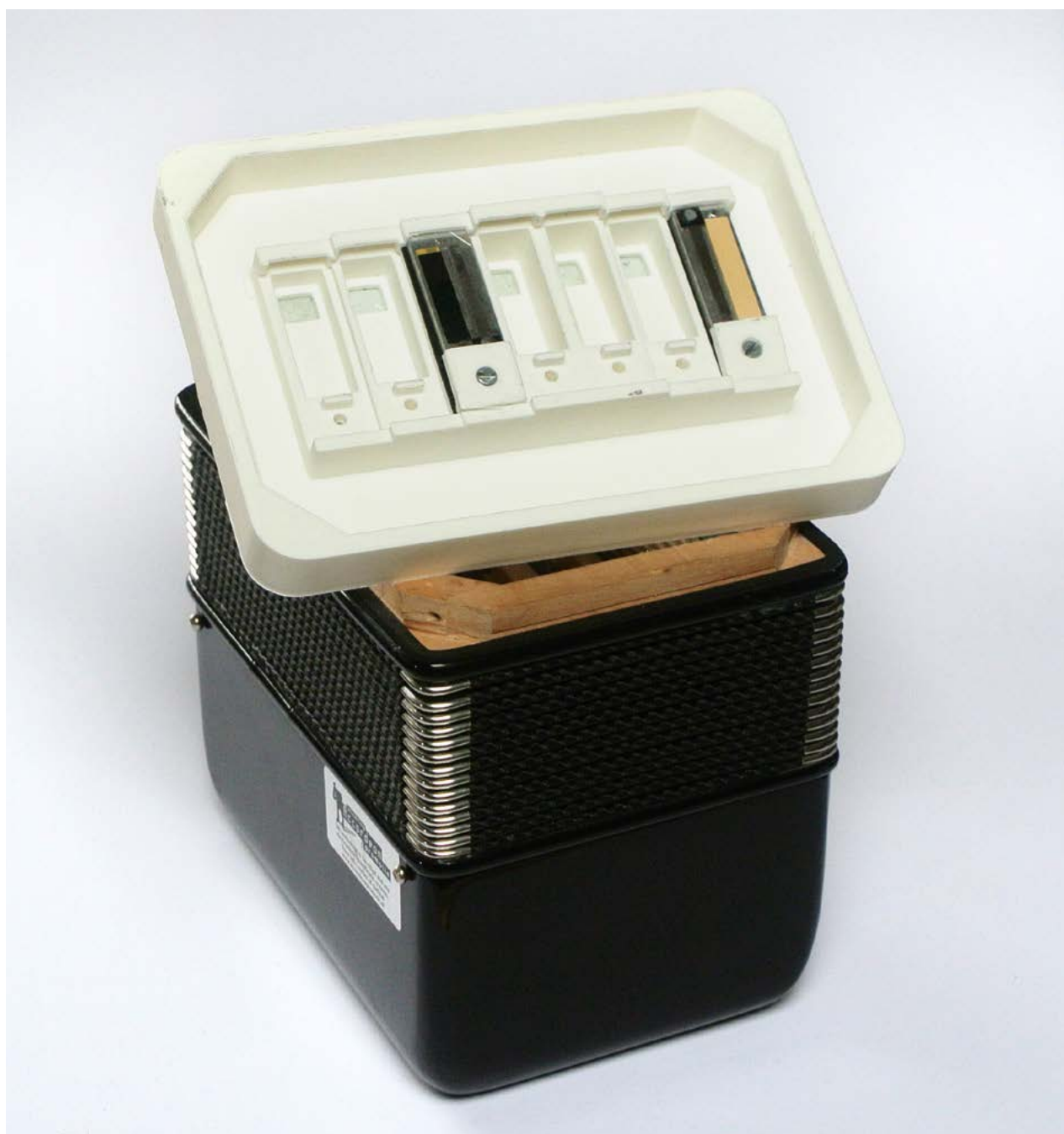
The reeds are mounted on a different sound chamber for each recording
