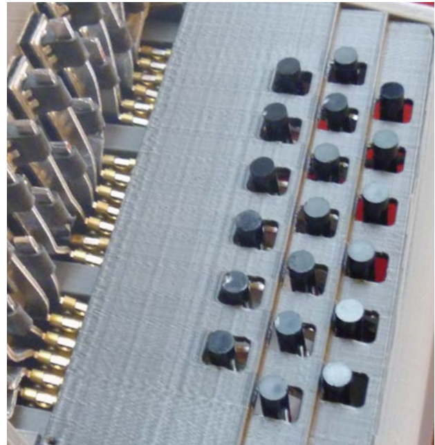
In order to take the button cover off for repairs, all buttons need to be removed from their cylindrical base, since they form an obstruction.
