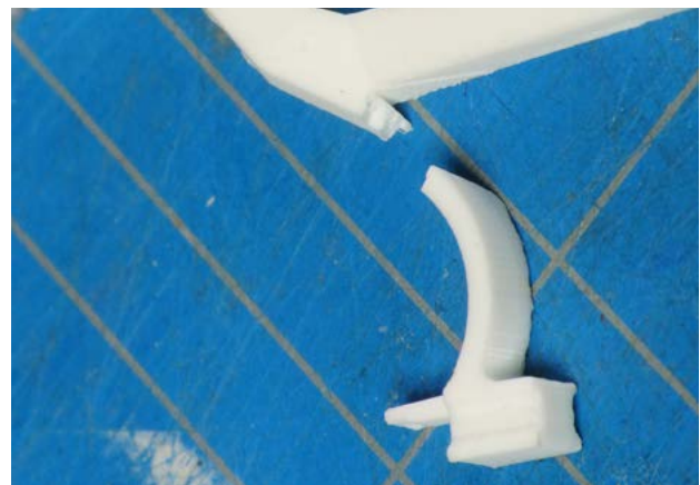
The result of test 2: a completely destroyed spring
