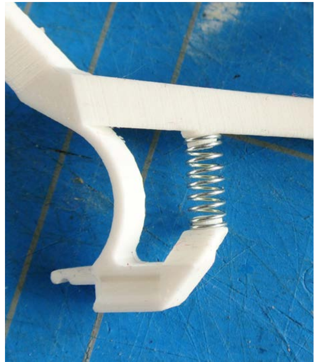
The new spring position, placed here on a impractical plateau
