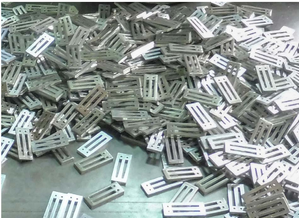
Aluminium reed housings are produced using a punch. Here, they await assembly of the reed.
