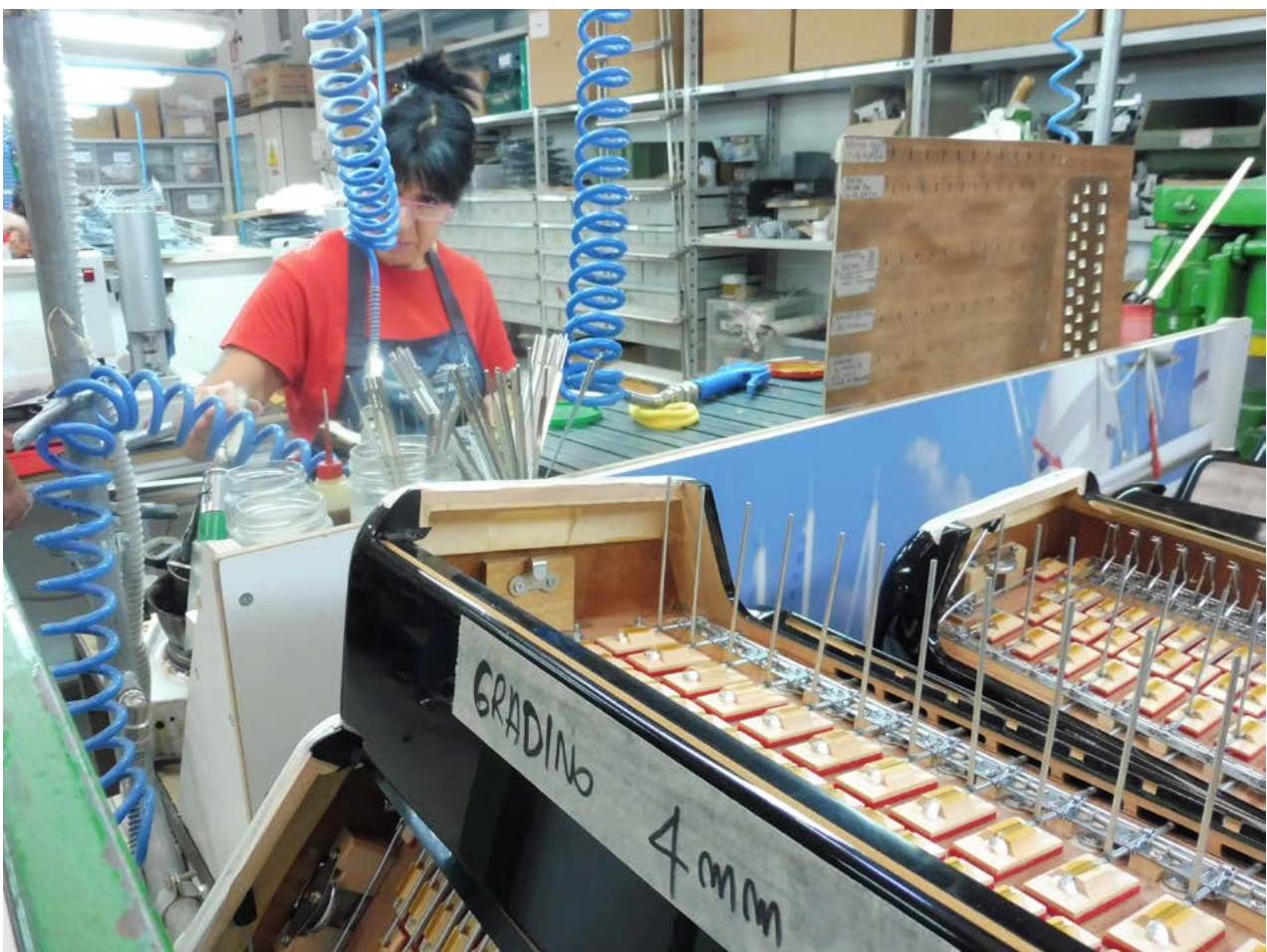
Custom components are written out on a layer of tape for the relevant production steps
