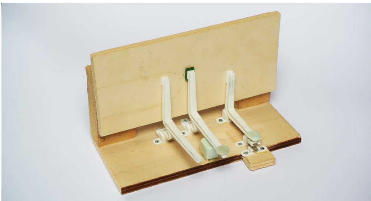
This model indicates the magnet system is suboptimal because of guiding problems. The printed spring designs perform well.
