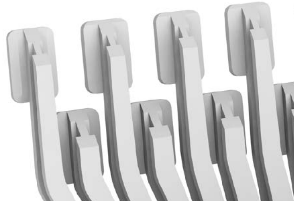
The first design of the valve pads is dimensionally suboptimal
