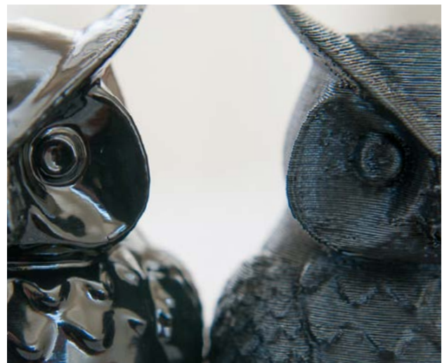
The ABS FDM print on the left has been smoothed using acetone vapour.
