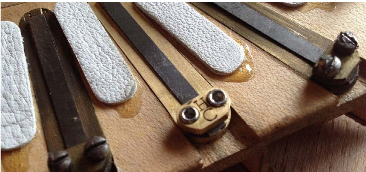
Concertina reeds, mounted in a slot using a form closure
