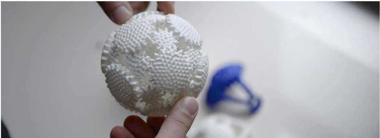
A ball of gears like this could not be produced without additive manufacturing techniques
