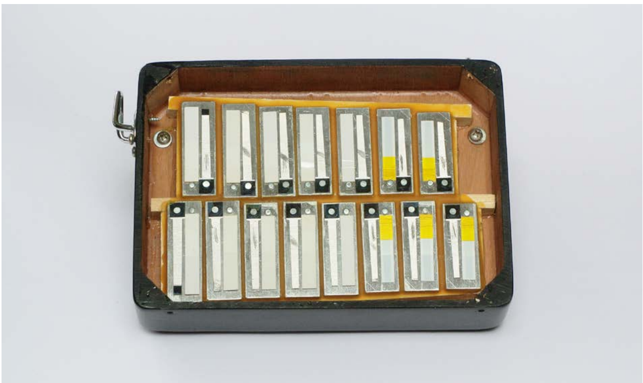
A finished conventional instrument, using wax to attach the reeds
