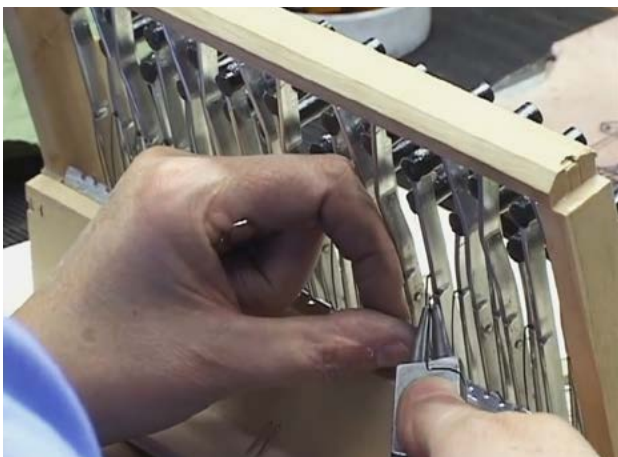
Placing the torsion springs in the arms
