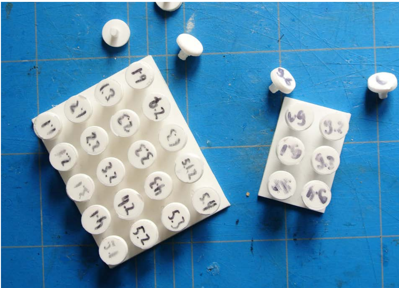
Subtle dimensional variations of snap fit design are used to determine the correct fit
