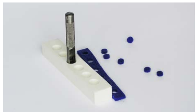
Custom felt die and tools for punching holes
