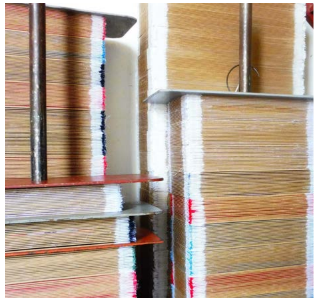
Bellows are pressurised to keep them in a closed position
