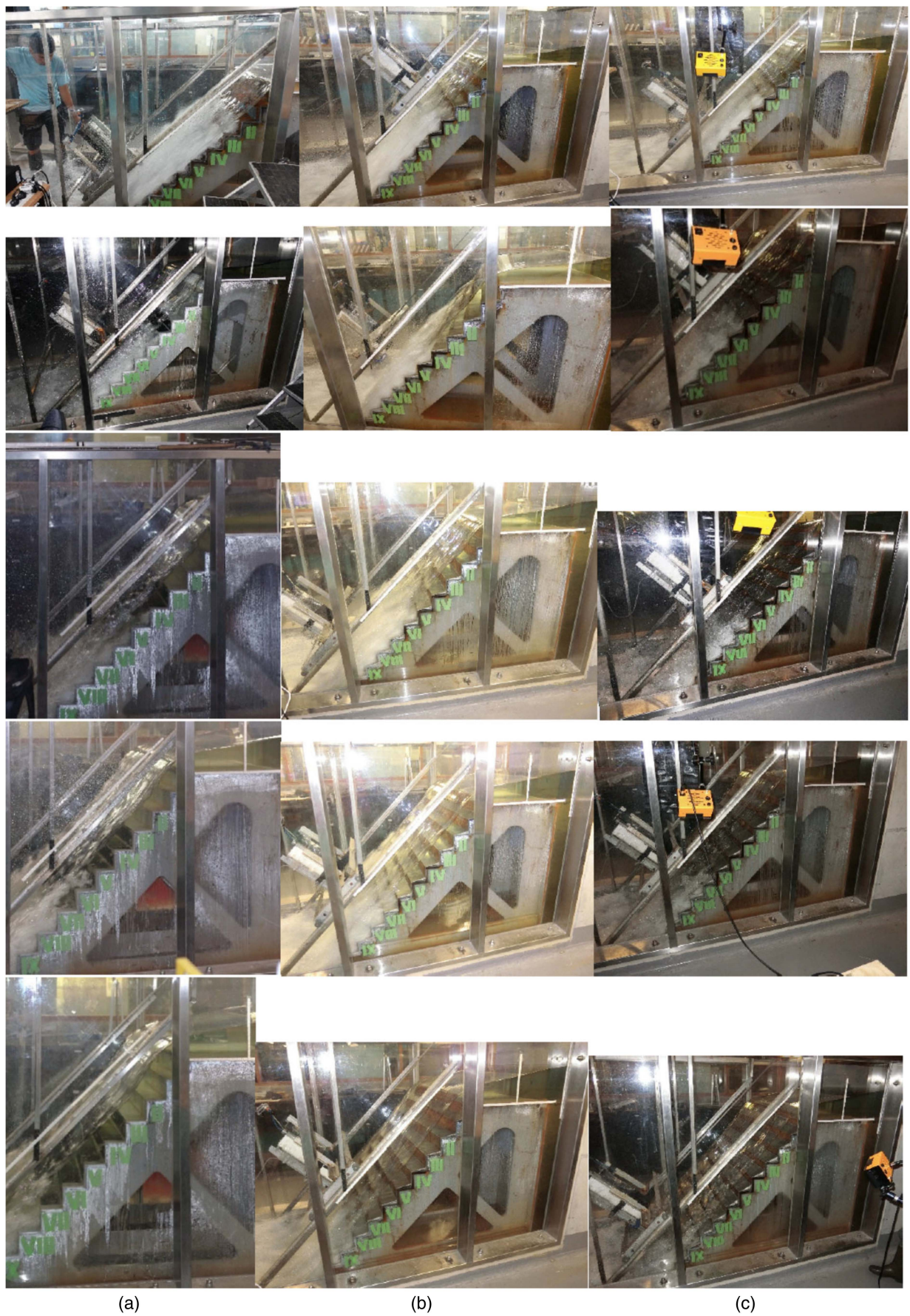
Fig. 4. Effects of the dimensionless discharge on 45° stepped chute with horizontal and inclined steps. From top to bottom: d_c/h = 0.8, 1.0, 1.2, 1.4, and 1.6 : (a) flat horizontal steps ( \delta = 0 and \lambda/k = 2.0 ); (b) 1V:5H inclined steps ( \delta = 11.3^\circ and \lambda/k = 2.5 ); and (c) 1V:2.3H inclined steps ( \delta = 23.3^\circ and \lambda/k = 3.0 ).
