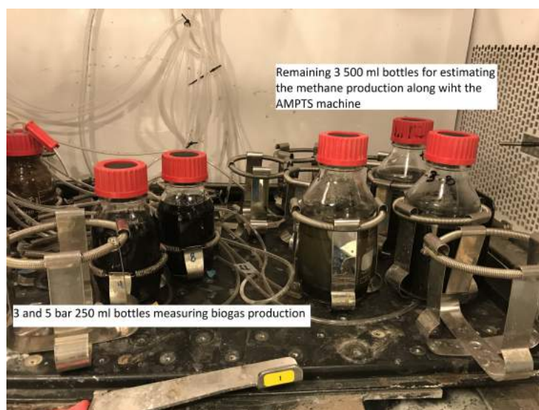
Figure 3.5: Samples for methane production (3 - 500 ml bottles) and for biogas production (2 -250 ml bottles) in the incubator shaker.
