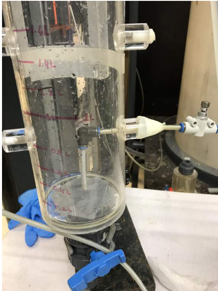
Figure 4.9: Pictorial representation of the mechanism of aeration inlet in the lab setup
