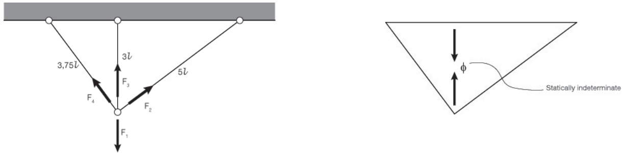
fig. 2.15 a force F_1 on a node supported by three bars
