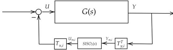
Figure 3.3.: The block diagram for close-loop interconnection
