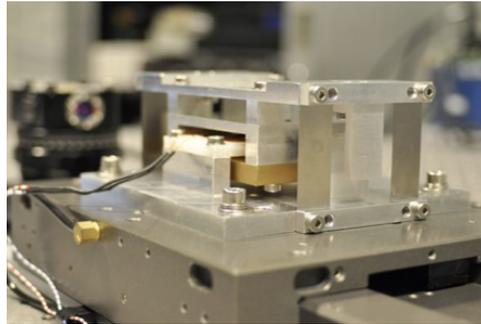
Figure 1.1.: Motion stage with parallel leaf spring
