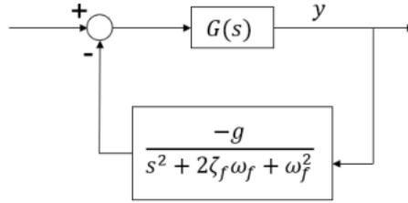
Figure 2.7.: Principle of Positive Position Feedback [9]
