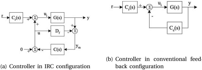
Figure 2.5.: Integral resonant control [5]
