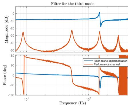
Figure 4.2.: Online implementation of  $T_{u,3}$  and  $T_{y,3}$
