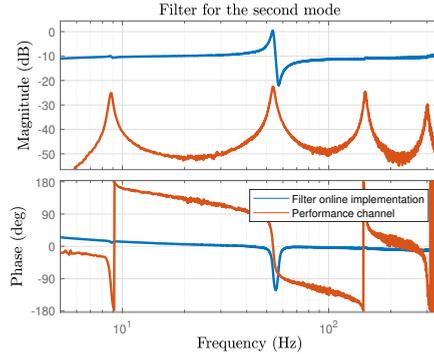
Figure 4.1.: Online implementation of  $T_{u,2}$  and  $T_{y,2}$
