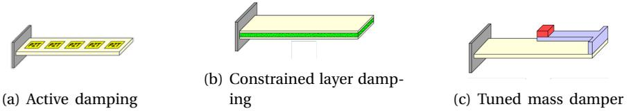
Figure 1.2.: Different damping methods [3]
