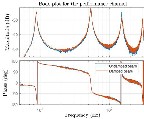
Figure 4.5.: Frequency response of the performance channel
