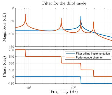
Figure 4.7.: Offline simulation of  $T_{u,3}$  and  $T_{y,3}$
