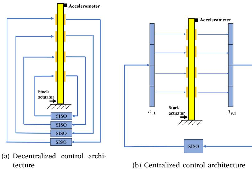
Figure 1.4.: Decentralized and centralized control architecture
