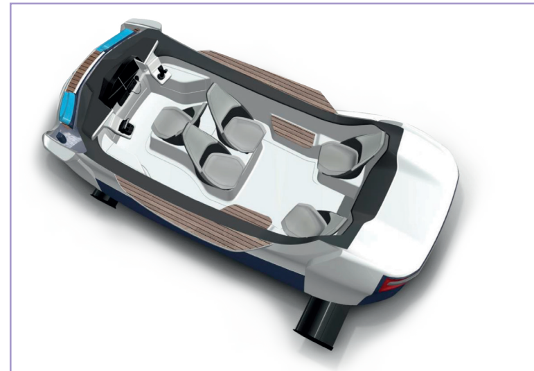
FIGURE 19 The interior set-up of the Seabubble
