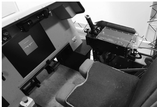
Figure 6. Fixed-base simulator setup, showing the visual display and the electro-hydraulic servo-controlled sidestick.
