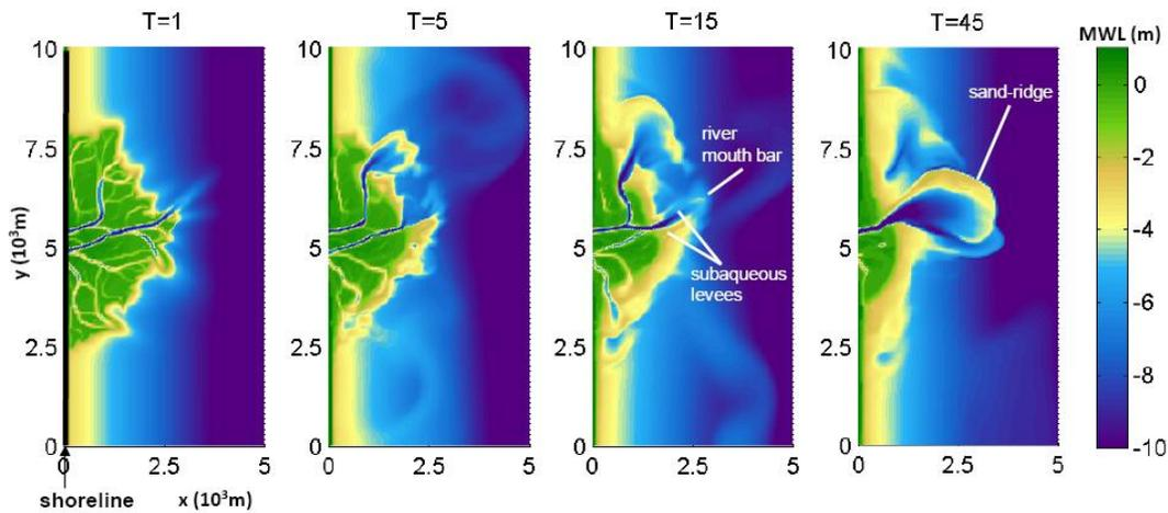
Figure 5.23 Plan view morphology for fluvial input simulation #4 (discharge 2,000 m<sup>3</sup>/s, equilibrium sediment supply) over time
