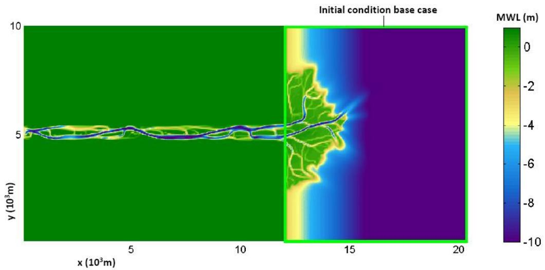
Figure 4.1 Plan view morphology of reference model including river system with the initial condition of the base case highlighted
