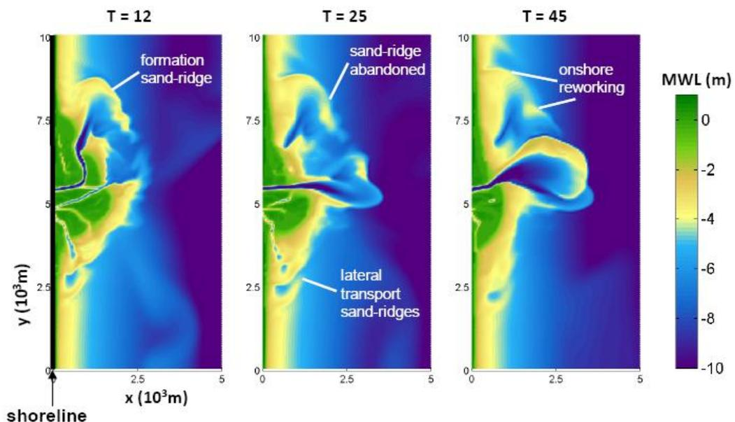
Figure 5.36 Formation and reworking of sand-ridges in fluvial input simulation #4
