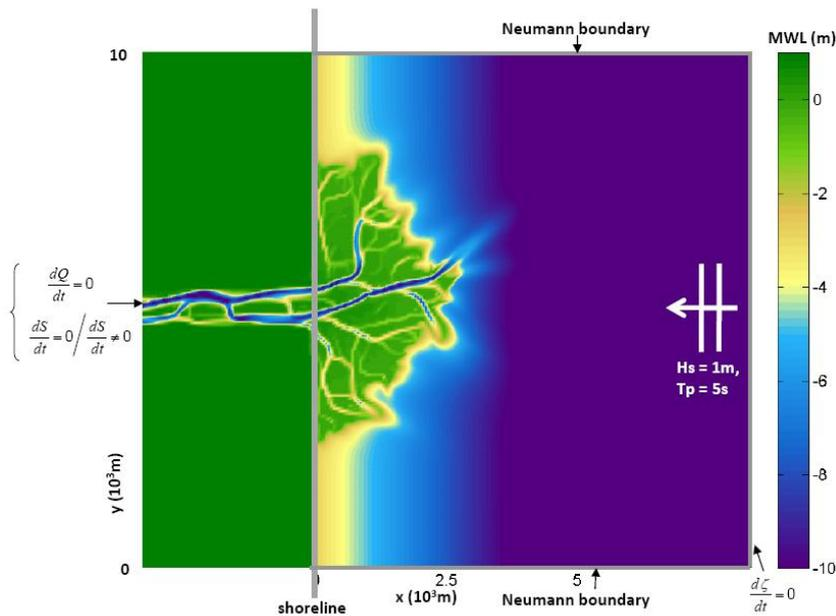
Figure 4.6 Model schematization fluvial input case
