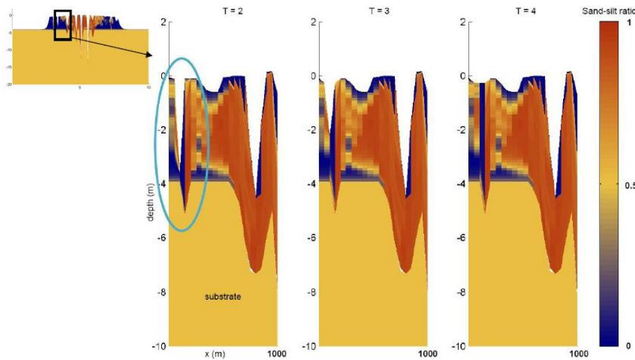
Figure 5.10 Process of distributary infill by fine silt, detail of cross-section M-M'
