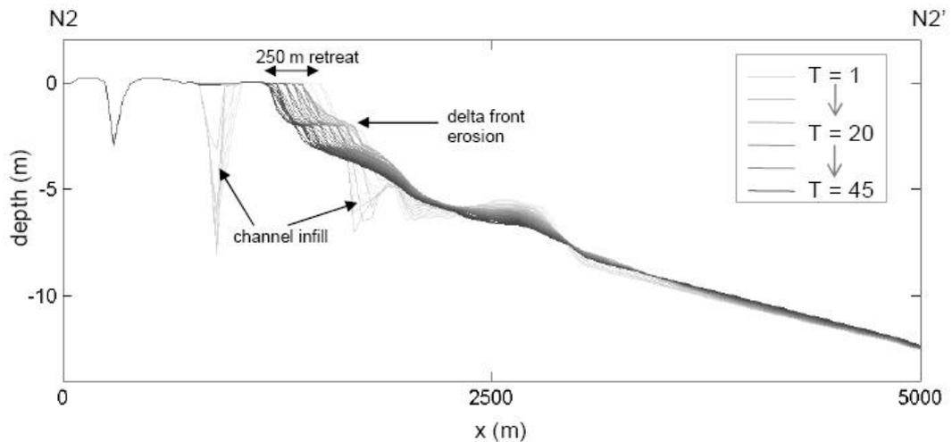
Figure 5.8 Bed profiles of crossshore cross-section N2-N2' over time
