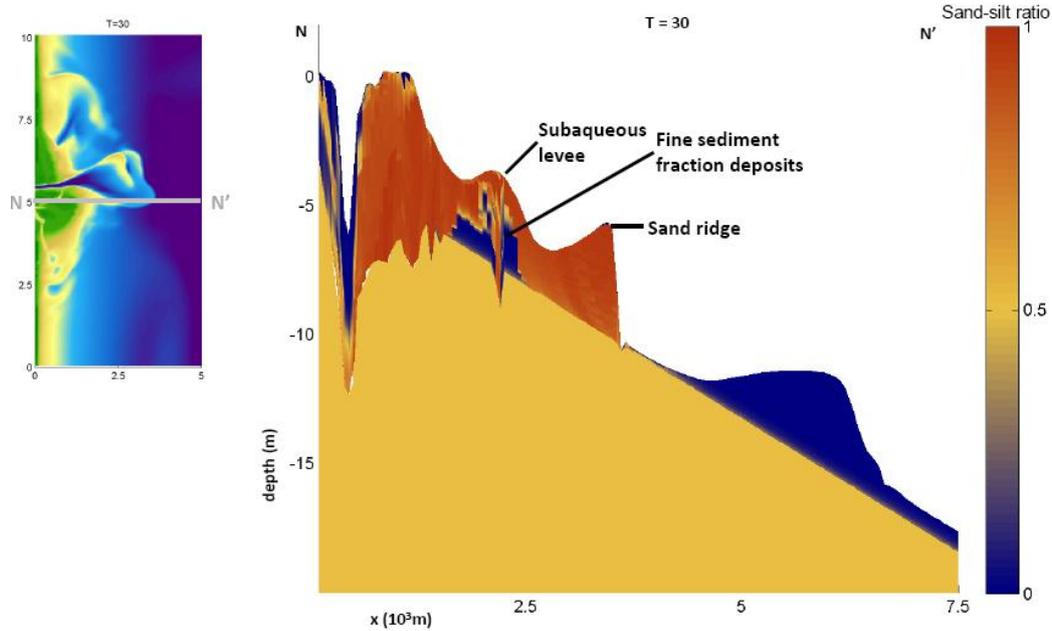
Figure 5.31 Crossshore stratigraphic cross-section illustrating partial preservation of fine sediments topped by sand deposition
