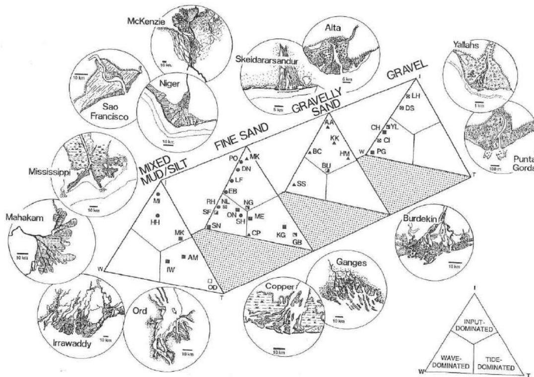
Figure 2.8 Diagram of delta classification based on dominant processes (input, wave or tide) and grain size (Orton and Reading, 1993)
