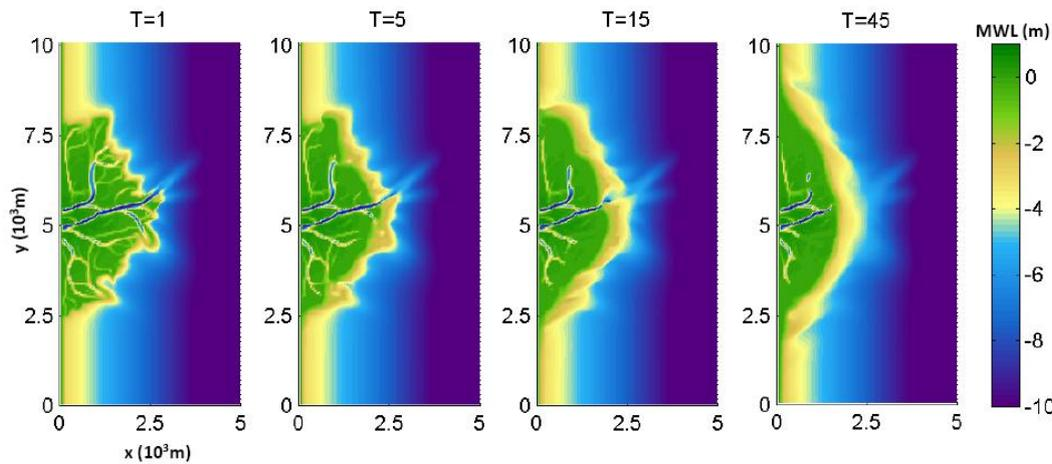
Figure 5.43 Plan view morphology over time of sensitivity run with both sediment fractions with the same characteristics
