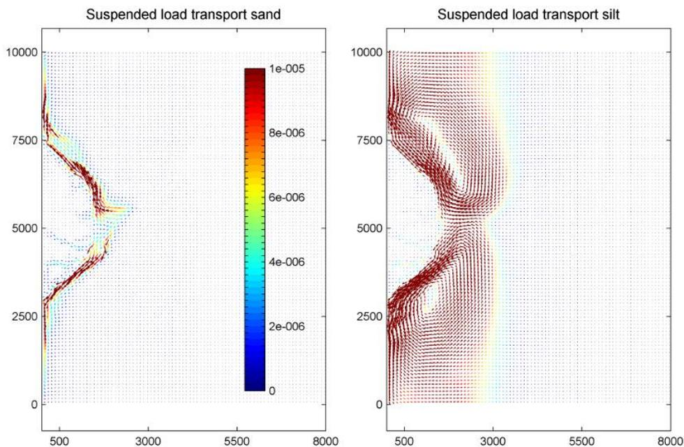
Figure 5.14 Mean suspended load transport of sand fraction (left) and silt fraction (right)
