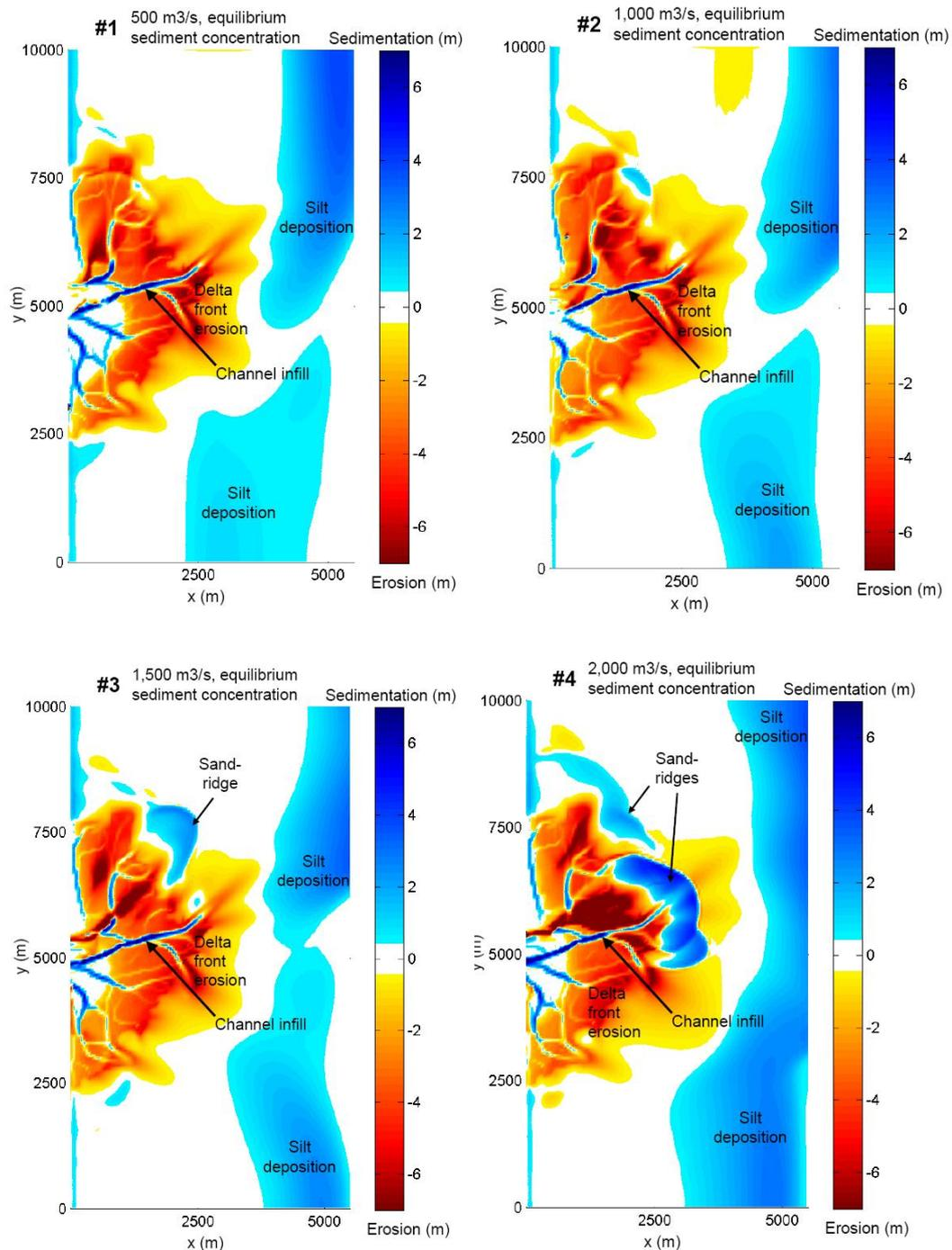
Figure 5.27 Cumulative sedimentation and erosion patterns simulations (#1, 2, 3 and 4) of fluvial input case
