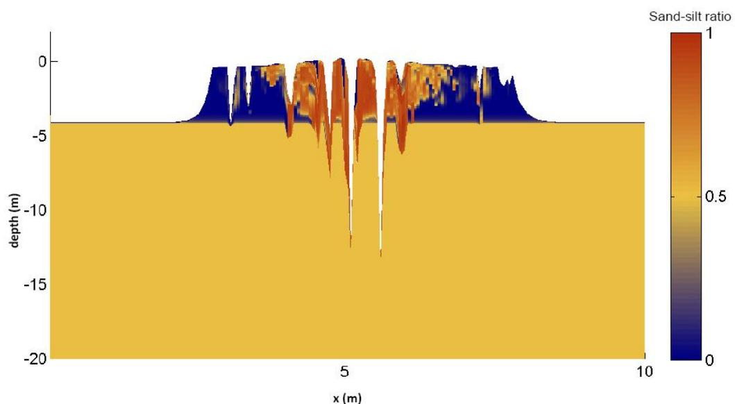
Figure 5.3 Stratigraphy (ratio sand – silt) initial condition of longshore cross-section M-M'
