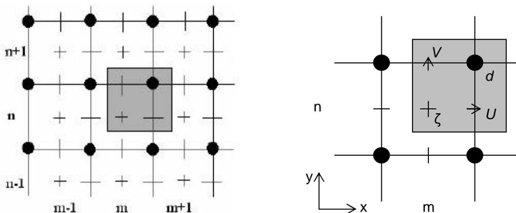
Figure 3.2 Staggered grid of Delft3D (Deltares, 2007a) (left) and staggered grid as used in this project (right)
