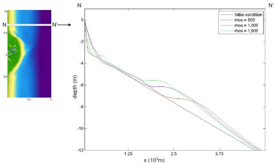
Figure 5.42 An overview of the resulting crossshore profiles ( $N=170$ ) with different dry bed densities of the fine sediment fraction
