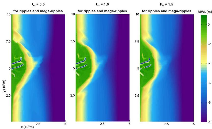
Figure 5.46 Overview of resulting morphology of the sensitivity tests with different bed form factors
