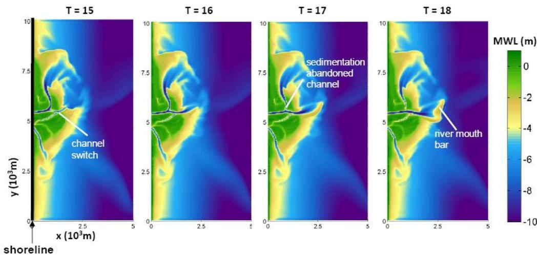
Figure 5.35 Process of channel switching and sedimentation of abandoned channel for fluvial input simulation #8
