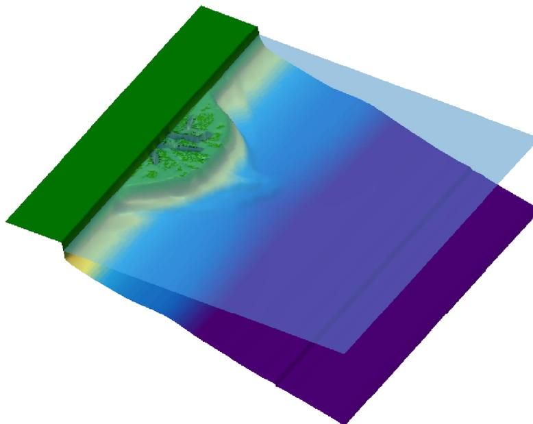
Figure 5.5 3D representation of the resulting morphology of the base case
