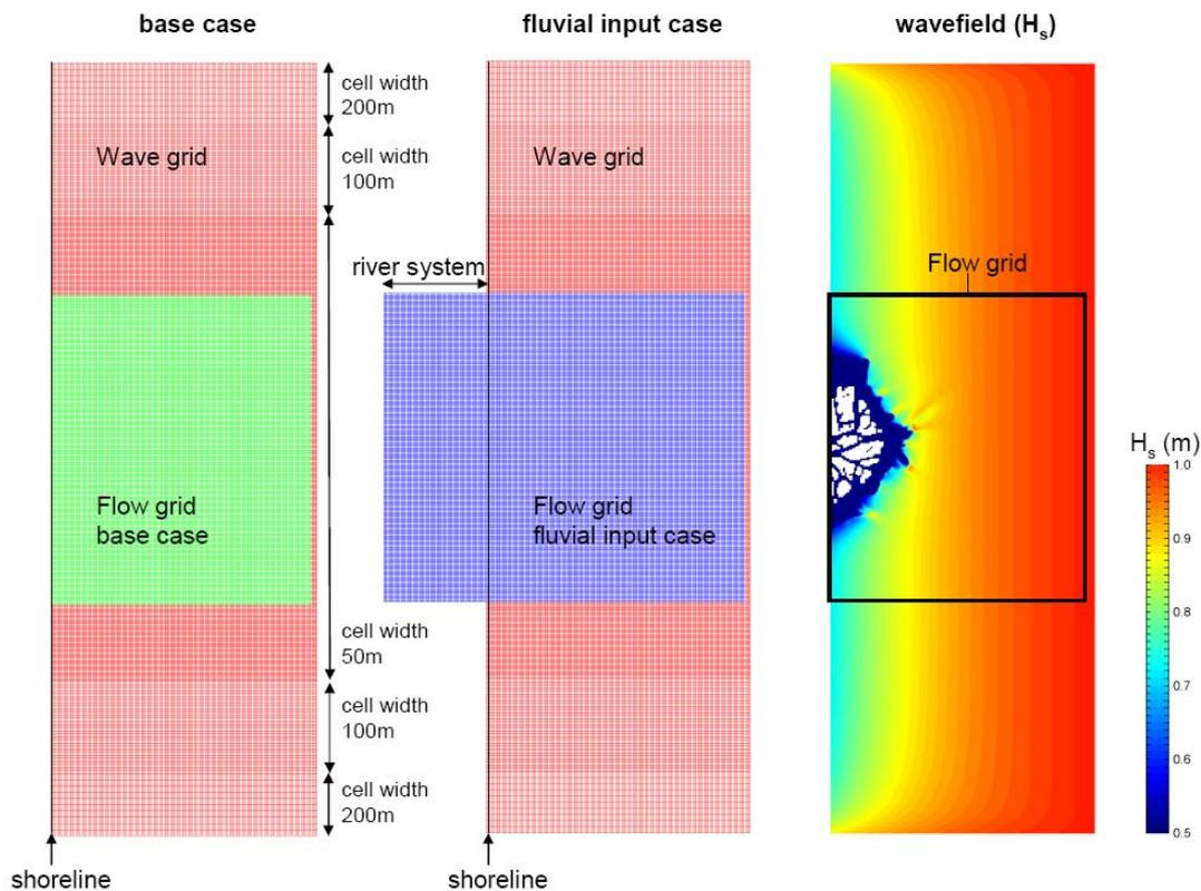
Figure 4.4 Wave and Flow grids of the base case and fluvial input case and significant wave height of wave field
