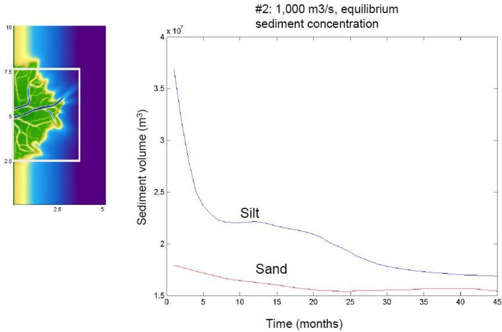
Figure 5.28 Sediment budget of deltaic environment, as indicated in the insert, showing the decrease of sediments over time for simulation #2 of the fluvial input case
