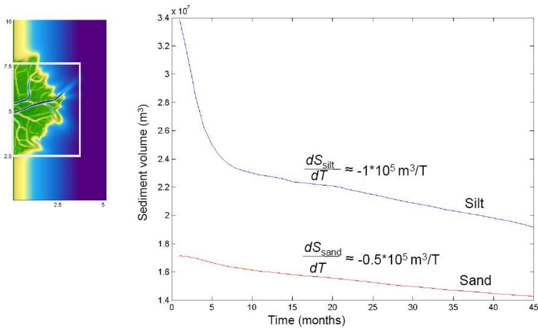
Figure 5.17 Sediment budget of deltaic environment, as indicated in the insert, showing the decrease of sediments over time
