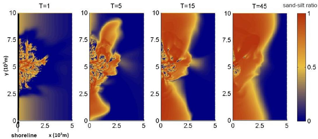
Figure 5.26 Plan view of the grain size distribution in the transport layer of fluvial input case simulation #4
