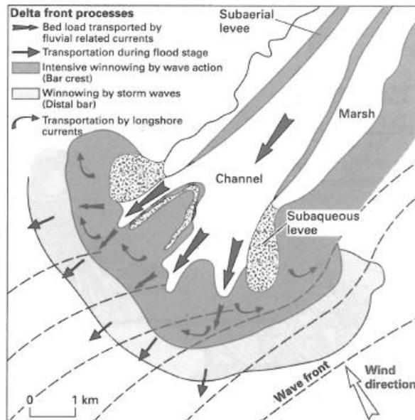
Figure 2.18 Delta front processes (Coleman and Gagliano, 1965 adjusted by (Reading and Collison, 1996))
