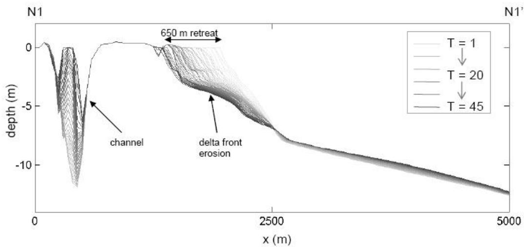
Figure 5.7 Bed profiles of crossshore cross-section N1-N1' over time
