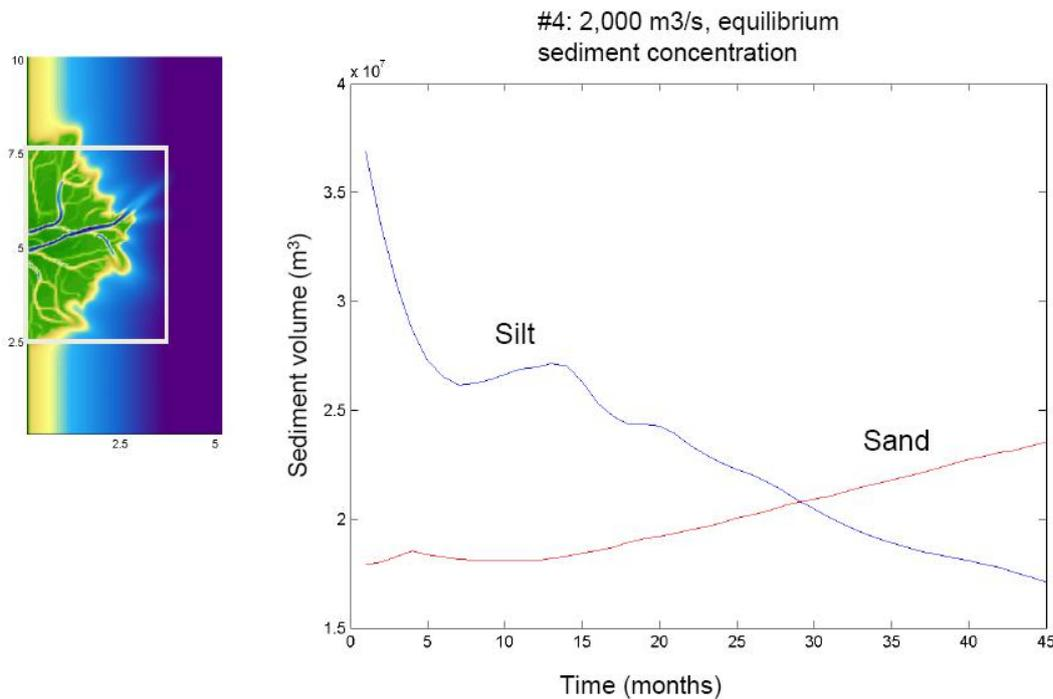
Figure 5.29 Sediment budget of deltaic environment, as indicated in the insert, showing the decrease of sediments over time for simulation #4 of the fluvial input case
