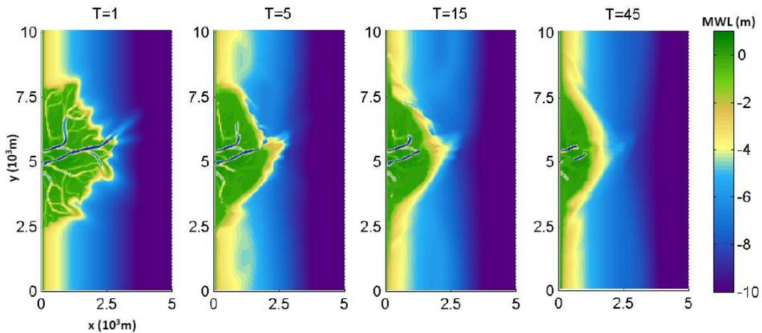
Figure 5.44 Plan view morphology over time of sensitivity run with friction determined with Chézy ( $C= 60 \text{ m}^{1/2}/\text{s}$ )
