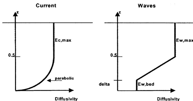
Figure 3.5 Vertical distribution of sediment mixing coefficients (van Rijn, 2007b)
