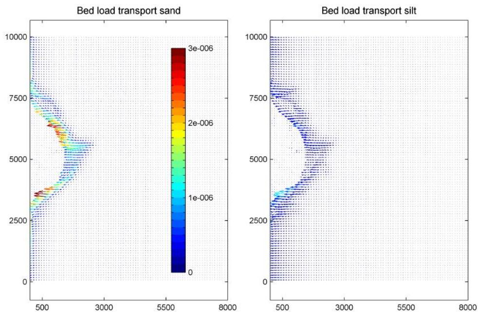
Figure 5.12 Mean bed load transport of sand fraction (left) and silt fraction (right)
