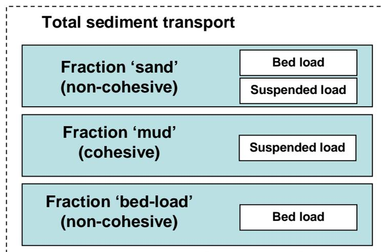
Figure 3.3 Schematic overview of sediment transport via different sediment fractions in Delft3D-Flow
