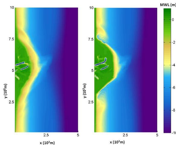
Figure 5.38 Plan view of resulting morphology of sensitivity runs with different wave-related bed load transport factors
