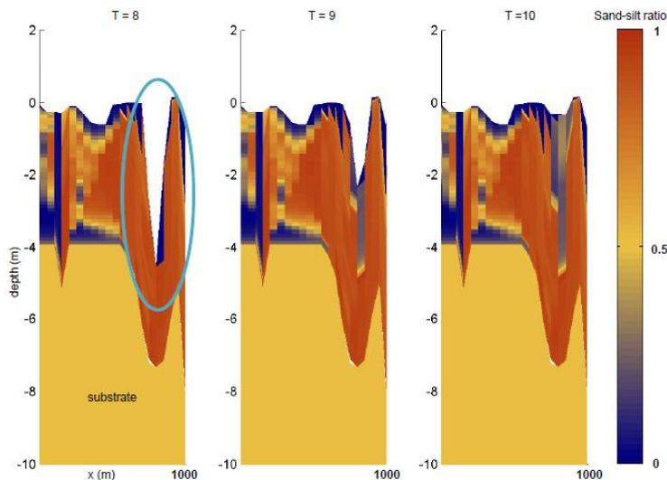
Figure 5.11 Process of distributary infill by fine silt, detail of cross-section M-M'
