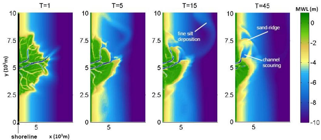
Figure 5.21 Plan view morphology for fluvial input simulation #1 (discharge  $500 \text{ m}^3/\text{s}$ , equilibrium sediment supply) over time
