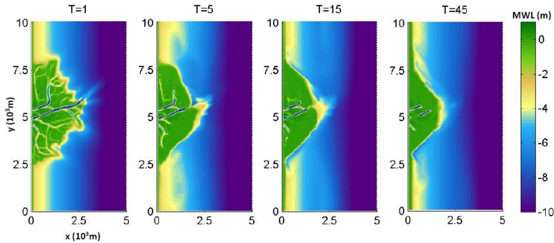
Figure 5.45 Plan view morphology over time of sensitivity run with friction determined with Manning ( $n = 0.03 \text{ m}^{-1/3}/\text{s}$ )
