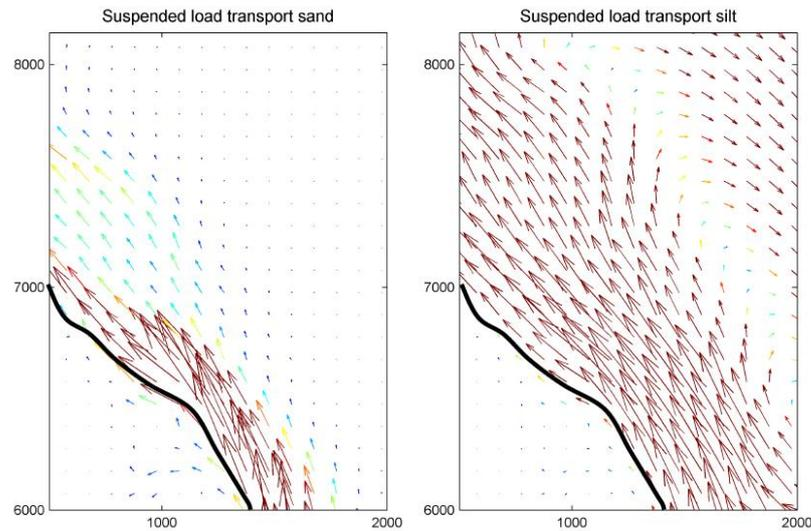
Figure 5.15 Details of mean suspended load transport of sand fraction (left) and silt fraction (right)
