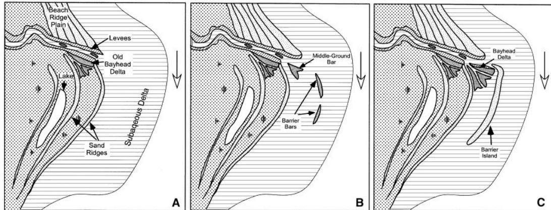
Figure 2.19 Wave-influenced delta evolution model, with subaqueous phase (A), middle-ground bar phase (B) and barrier island phase (C) (Bhattacharya and Giosan, 2003).
