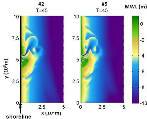
Figure 5.32 Resulting morphology of fluvial input simulations #2 and #5 with the same water discharge, with a different (but comparable) sediment boundary condition
