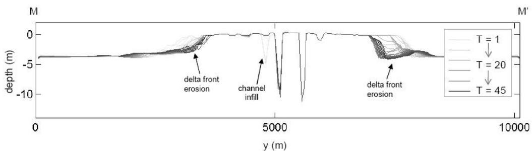
Figure 5.9 Bed profiles of longshore cross-section M-M' over time
