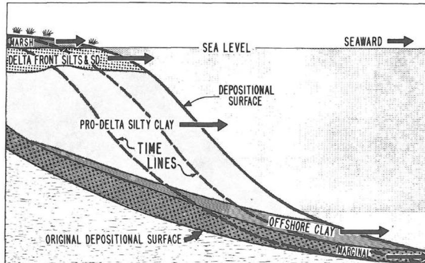
Figure 2.13 Constructional phase of a deltaic cycle (Scruton, 1960)
