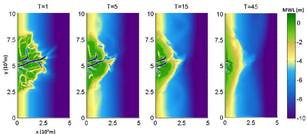
Figure 5.37 Plan view morphology over time of sensitivity run with no wave-related transports
