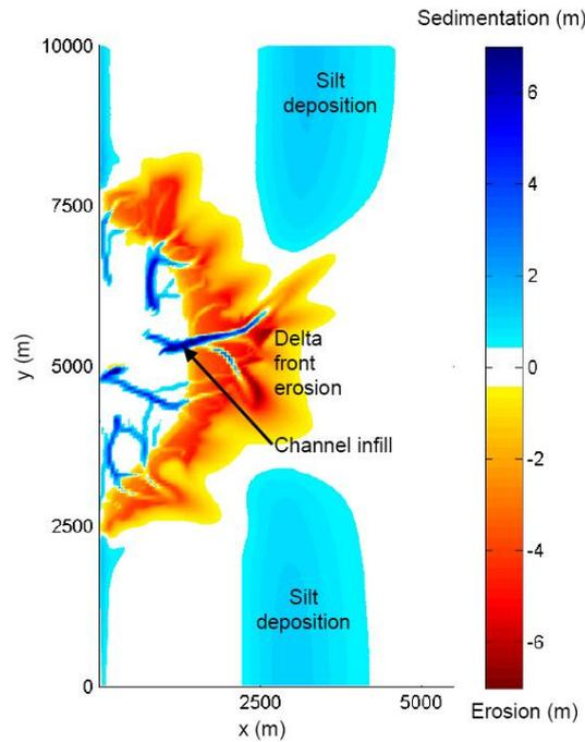
Figure 5.16 Plan view of cumulative sedimentation and erosion of the base case
