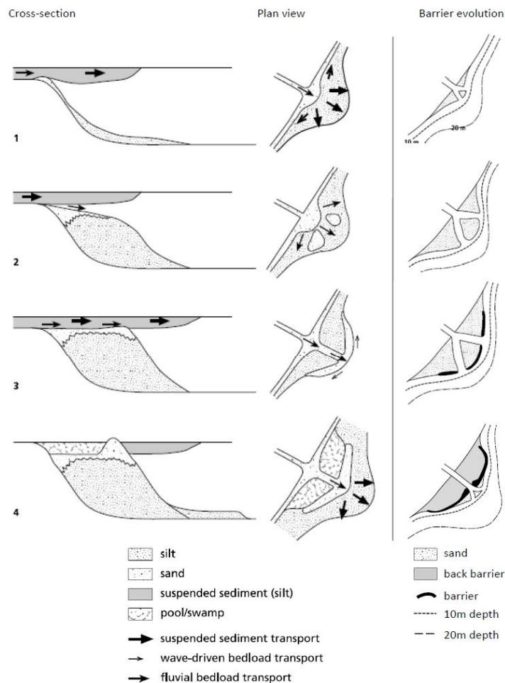
Figure 2.20 Cyclic delta growth (left) and barrier evolution (right) of the Ba Lat delta (van Maren, 2004)
