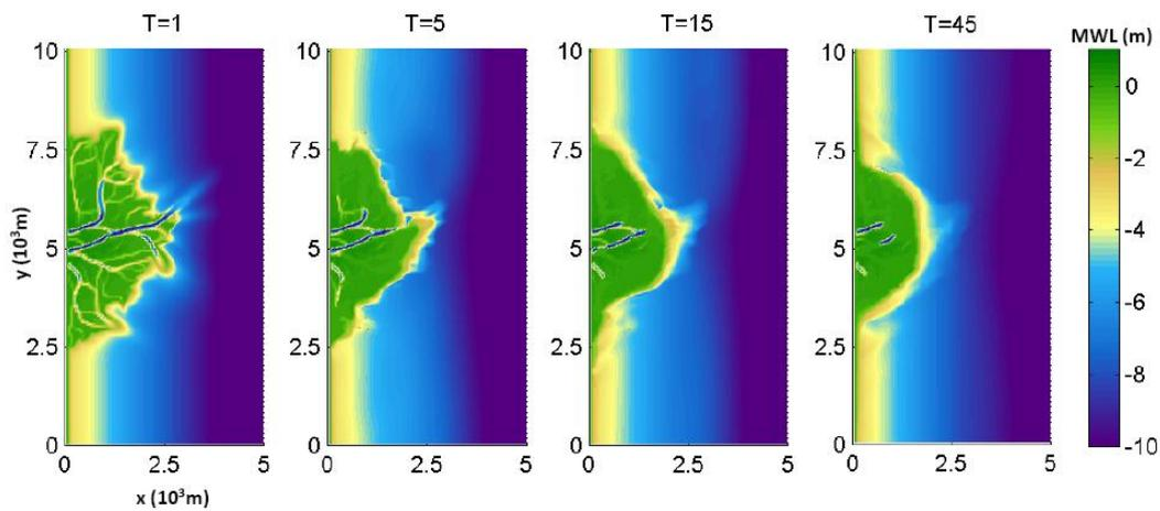
Figure 5.40 Plan view morphology over time of sensitivity run with  $d_{50}$  of the fine sediment fraction = 8  $\mu\text{m}$
