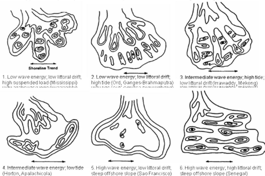
Figure 2.5 Six net sand distribution patterns resulting from combinations of control processes (Coleman and Wright, 1975).
