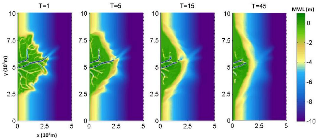
Figure 5.41 Plan view morphology over time of sensitivity run with  $d_{50}$  of the fine sediment fraction = 125  $\mu\text{m}$
