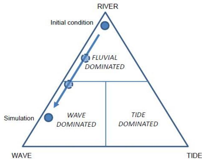
Figure 5.19 Change of dominant processes in the simulated deltaic environment based on the classification of Galloway (1975)
