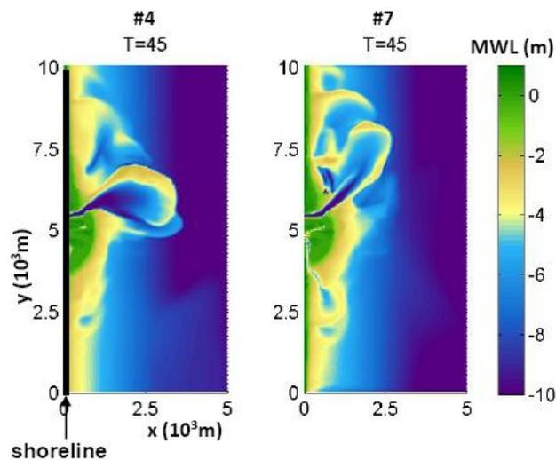
Figure 5.33 Resulting morphology of fluvial input simulations #4 and #7 with the same water discharge, with a different (but comparable) sediment boundary condition
