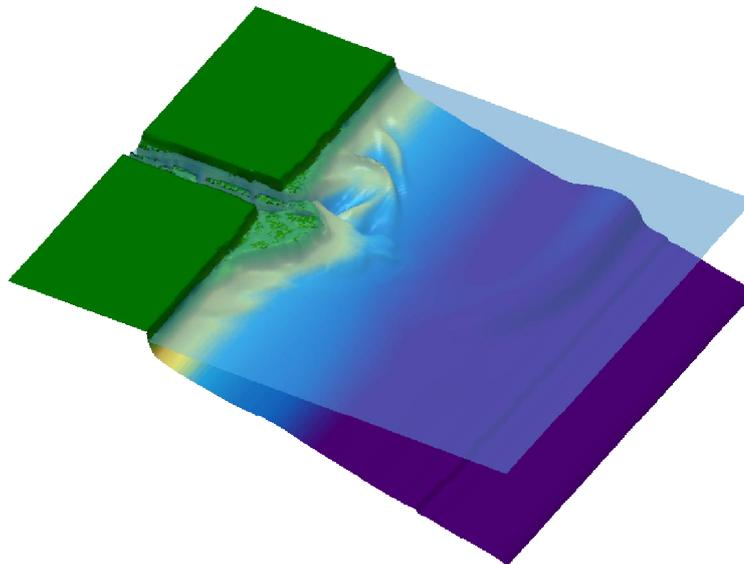
Figure 5.22 3D representation of the resulting morphology of fluvial input simulation #1
