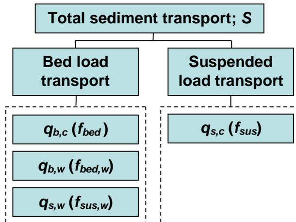
Figure 3.4 Schematic overview sediment transport and sediment transport coefficients
