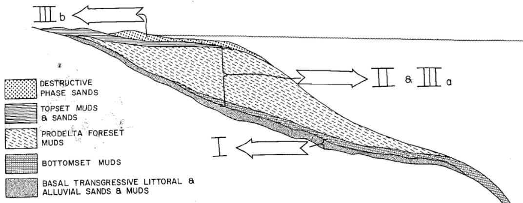
Figure 2.14 Constructional and destructional phase of delta (Curray, 1964)
