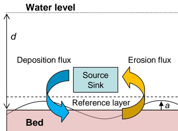
Figure 3.7 Schematic representation of the flux bottom boundary condition (adjusted after (Deltares, 2007a))
