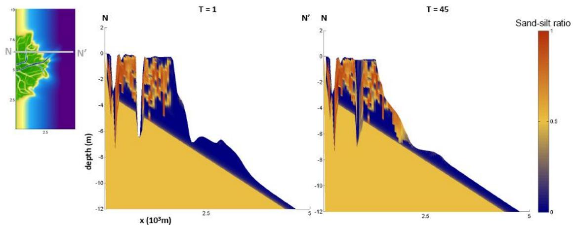
Figure 5.18 Crossshore stratigraphic sections ( $N = 125$ ) of initial and resulting condition to illustrate sediment sorting and shielding
