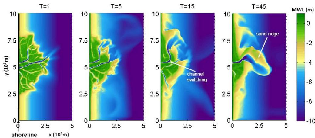
Figure 5.34 Plan view morphology of fluvial input simulation #8 over time
