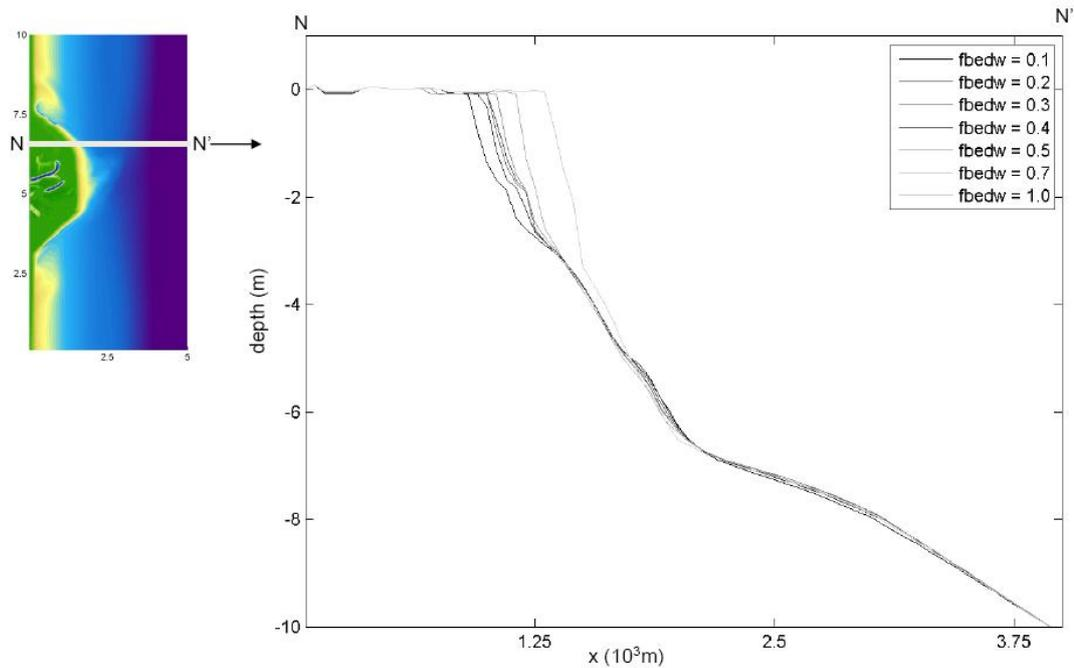
Figure 5.39 An overview of the resulting crossshore profiles ( $N=130$ ) with different wave-related bed load transport factors
