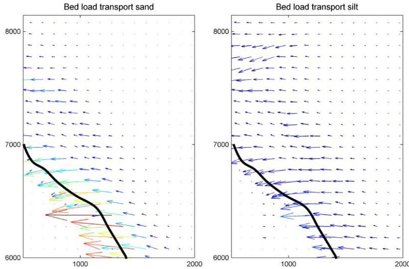
Figure 5.13 Details of mean bed load transport of sand fraction (left) and silt fraction (right)
