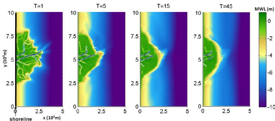
Figure 5.4 Plan view of morphology of deltaic environment of base case over time
