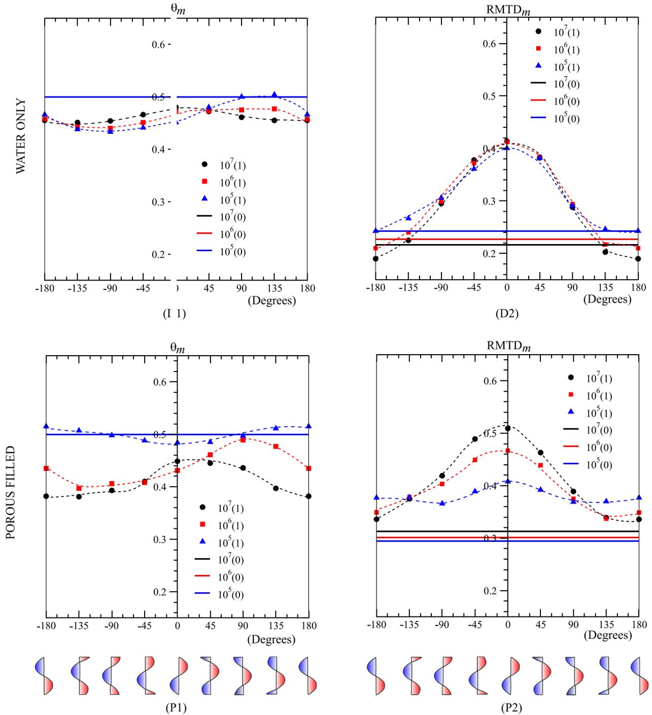
**Fig. 10.** Variation of non-dimensional volume-averaged mean temperature (D1, P1) and  $RMTD_m$  (D2, P2) of the fluid, with phase angle at different Rayleigh numbers ( $Ra_f = 10^5, 10^6, 10^7$ ) and different amplitudes (0, 1) of sinusoidal wall temperature in a water-only (top row) and porous media filled (bottom row) cavity. The dotted lines are only to guide the eyes.
