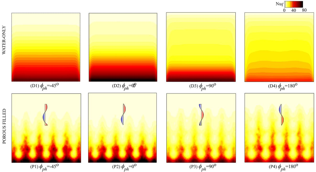
**Fig. 5.** Nusselt number contour at the right wall in a water-only (**top row**) and porous media filled (**bottom row**) cavity, with the left wall having sinusoidal temperature distribution of amplitude  $\theta_l^{amp} = 1$  and varying phase angle  $\Phi_{ph}$ , at  $Ra_f = 10^7$ . The contours are represented using a linear scale with 30 contour levels.
