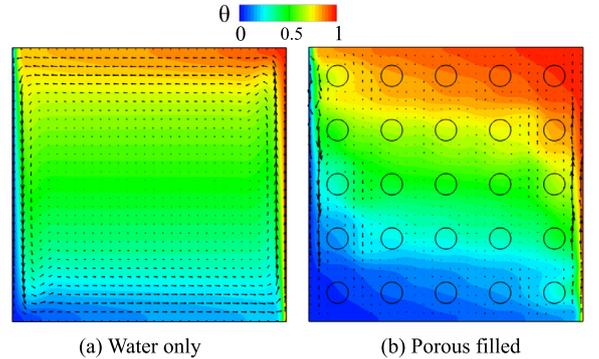
**Fig. 6.** Non-dimensional temperature contours and velocity vectors in a vertical plane at  $X/L = 0.41$  in a water-only (a) and porous media filled (b) cavity, with constant temperature  $\theta_l = 0$  and  $\theta_r = 1$ , at  $Ra_f = 10^7$ . The contours are represented using a linear scale with 30 contour levels.
