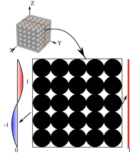
**Fig. 1.** Geometrical representation of the differentially heated water filled cavity with hydrogel beads. The left wall has a sinusoidal non-dimensional temperature, with mean value  $\bar{\theta}_l = 0$  and amplitude  $\theta_l^{amp} = 1$ ; and the right wall is maintained at a constant non-dimensional temperature  $\theta_r = 1$ .
