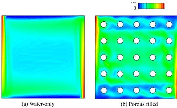
**Fig. 12.** Entropy generated due to temperature gradient in the fluid region (log scale) in a characteristic vertical plane at  $X/L = 0.41$  in a water-only (a) and porous media filled (b) cavity, with constant temperature left wall  $\theta_l = 0$  and right wall temperature  $\theta_r = 1$ , at  $Ra_f = 10^7$ .
