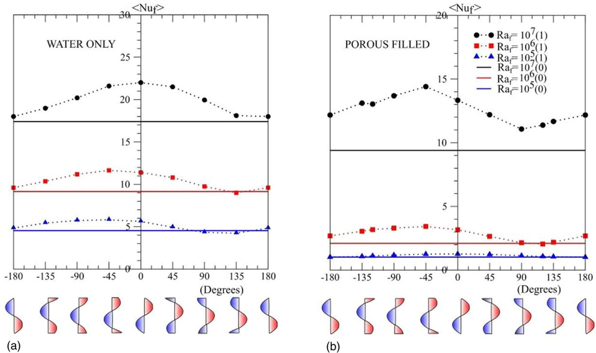
Fig. 2. Variation of wall-averaged Nusselt number with phase angle at different Rayleigh numbers ( $Ra_f = 10^5, 10^6, 10^7$ ) and different amplitudes,  $\theta_l^{amp} = 0$  (CWT), 1 in water-only (a) and porous media filled (b) cavity.
