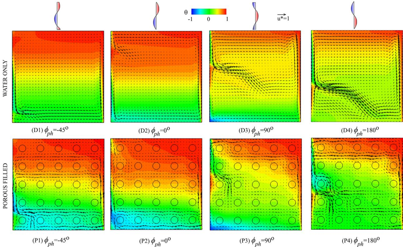
**Fig. 7.** Non-dimensional temperature contours and velocity vectors in a vertical plane at  $X/L = 0.41$  in a water-only (**top row**) and porous media filled (**bottom row**) cavities, with the left wall having a sinusoidal temperature distribution with amplitude  $\theta_1^{amp} = 1$  and varying phase angle  $\Phi_{ph}$ , at  $Ra_f = 10^7$ . The contours are represented using a linear scale with 30 contour levels.
