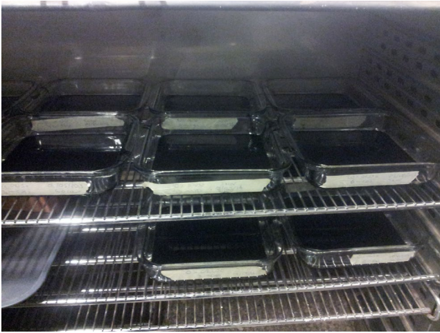
Figure 4. Binder-grape pomace mixes stored on a tray in a 60°C oven.
