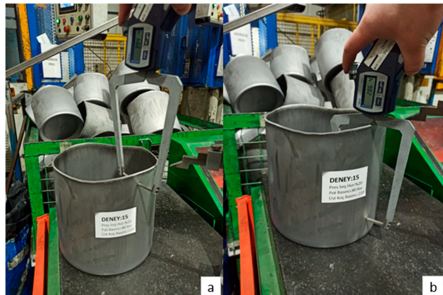
Figure 9. (a) Upper region thinning amount and (b) lower region thinning amount for Exp. 15.
