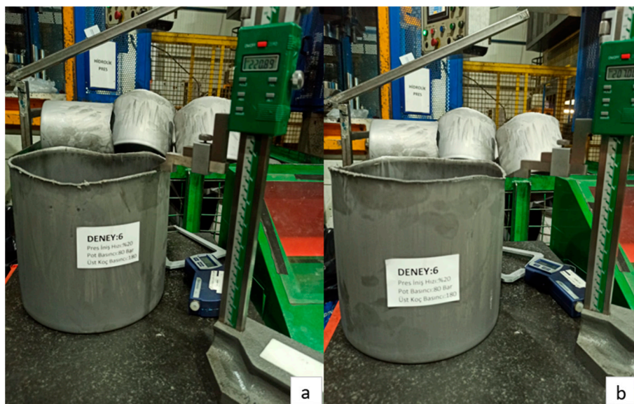
Figure 5. (a) Maximum elongation and (b) minimum elongation in Experiment 6.
