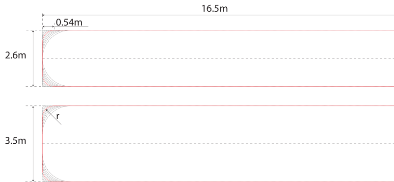
Figure 5.1: The GETS model and variations on the GETS model with different radii are shown. At the top a topview and in the middle a side view. The standard GETS model is shown in red, the variations are shown with a dashed line.
