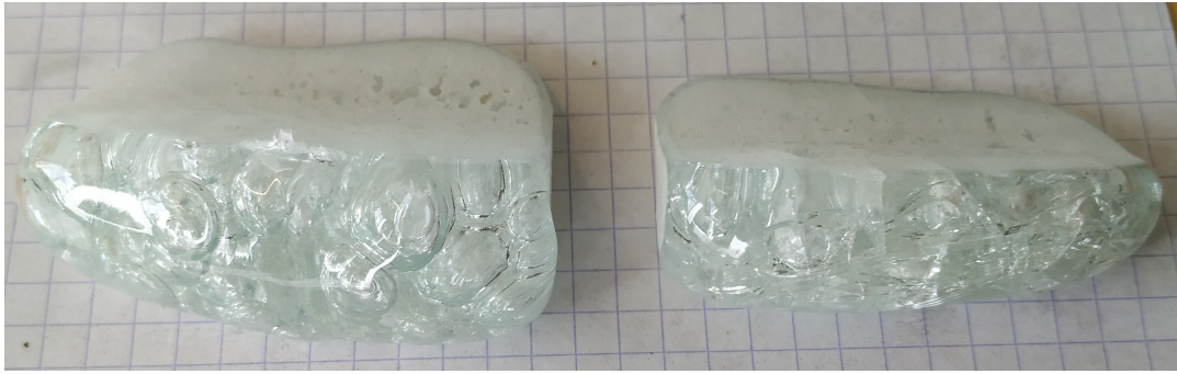
Figure D.0.2: Result of casting mixture IM-MOREC ( \sim 1600^\circ\text{C} ) onto preheated Crystal Cast ( \sim 1100^\circ\text{C} ).
