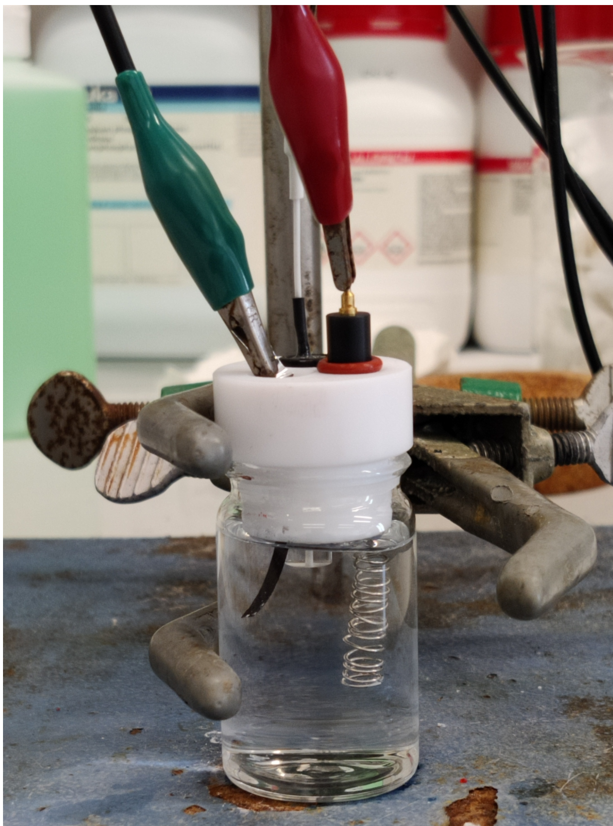
Figure 12: 3-electrode cell setup. Green is connected to the working electrode of the perylene-derivative and C45 aluminium strip. Red is connected to the platinum wire counter electrode; and white is connected to the Ag/AgCl reference electrode.
