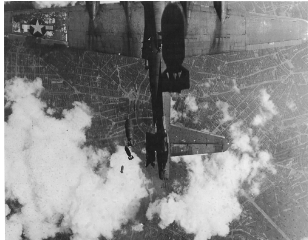
(b) Photograph 1 showing stabilizer after bomb impact.
