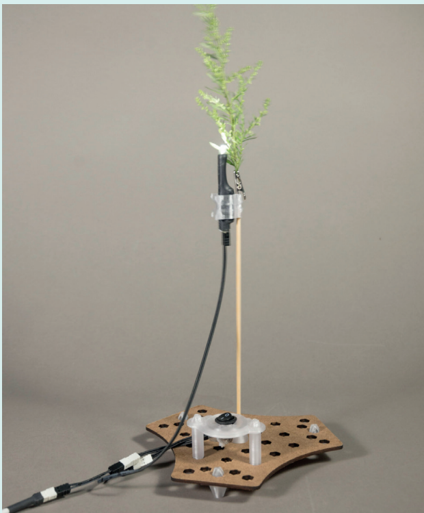
Figure 31: Vibration assembly. A vibration motor is connected to an on-off switch. (Dream Worlds, 2024)
