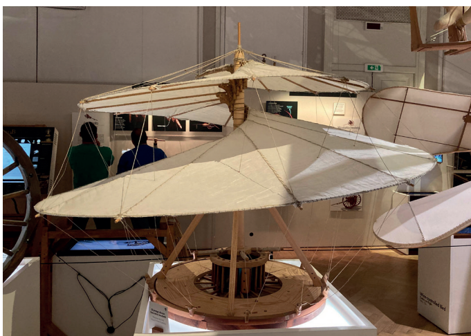
Figure 9: Aerial screw, model by Leonardo da Vinci (ca. 1485), reconstruction on display at Leonardo3 Museum, Milan.
