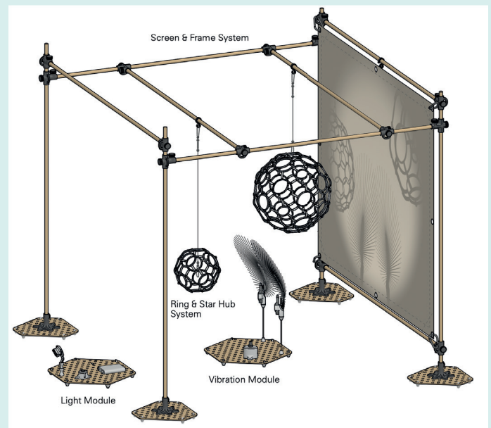
Figure 43: Final design of the screen and its frame. Allowing easy shadow play for the kit's users.
