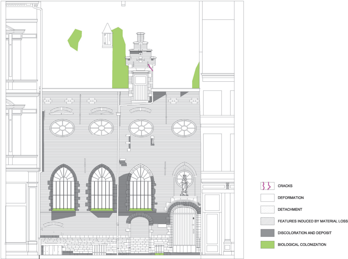
Figure 6: Map of state of conservation of applied materials, general assessment of the façade.
