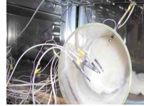
Picture 6-1: RV sensors in the glass tube
