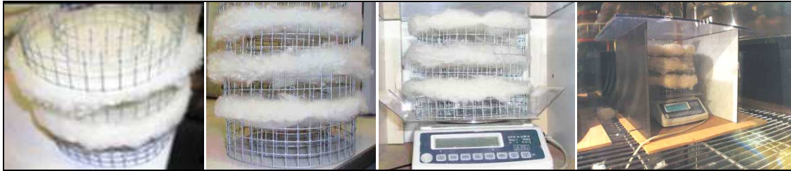
Picture 5-5: Wool specimen and the roster in between and the balance
