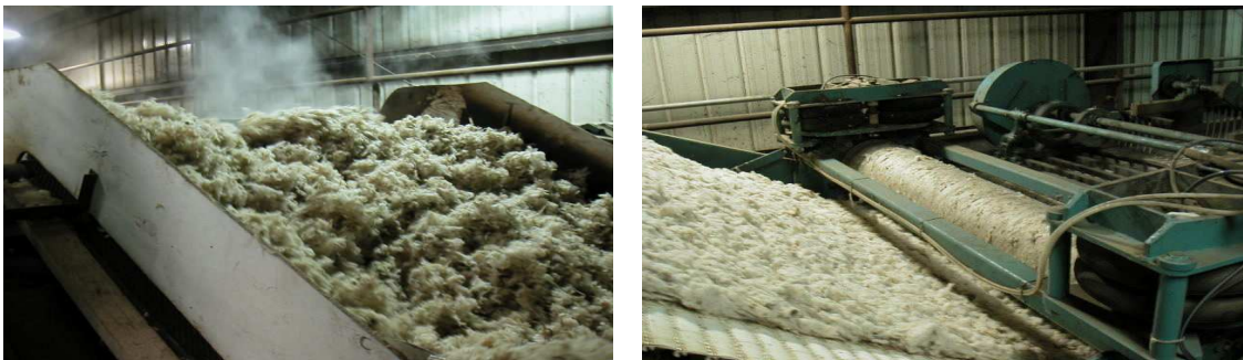
Picture 2-1: Scouring process of Sheep Wool
