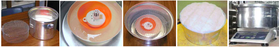
Picture 5-7: The set up of the water permeability experiment is shown step wise
