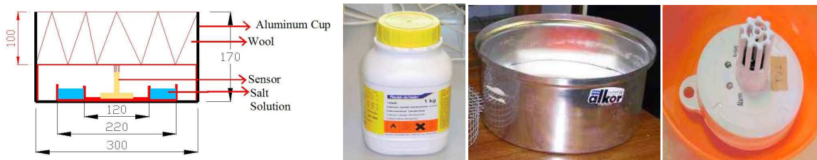
Picture 5-6: Schematic Drawing of the set-up, Salt ( \text{Ca}(\text{NO}_3)_2 \cdot 4\text{H}_2\text{O} ), Aluminum Cup and the Sensor
