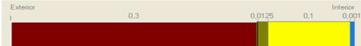
Figure 7-34 Insulated Closed Structure with Vapor Barrier
