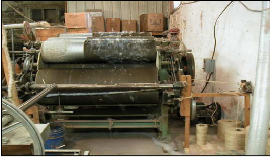
Picture 2-2: Carding Process after Scouring
