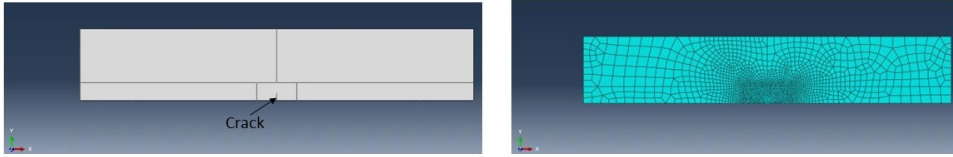
Figure 4.8: The dense mesh close to the crack and relatively sparse mesh in the other area of the FEM model
