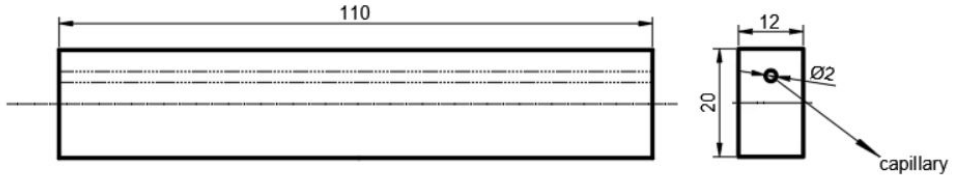
Figure 4.3: Nominal geometry of specimens used in four-point bending fatigue test
