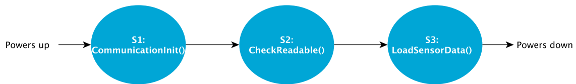
Figure 5.5: State diagram of the slave microcontroller
