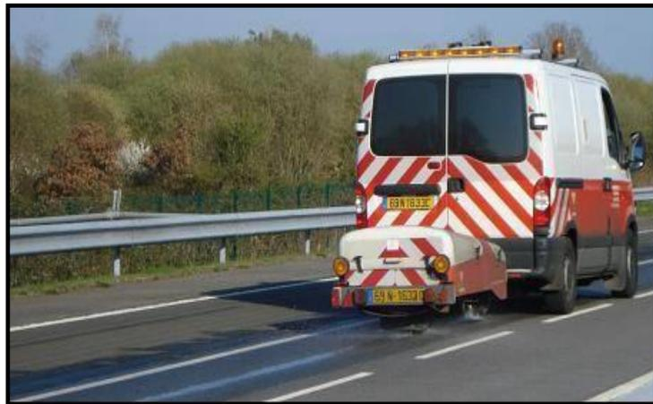
(c) Friction measurements by Adhera device
