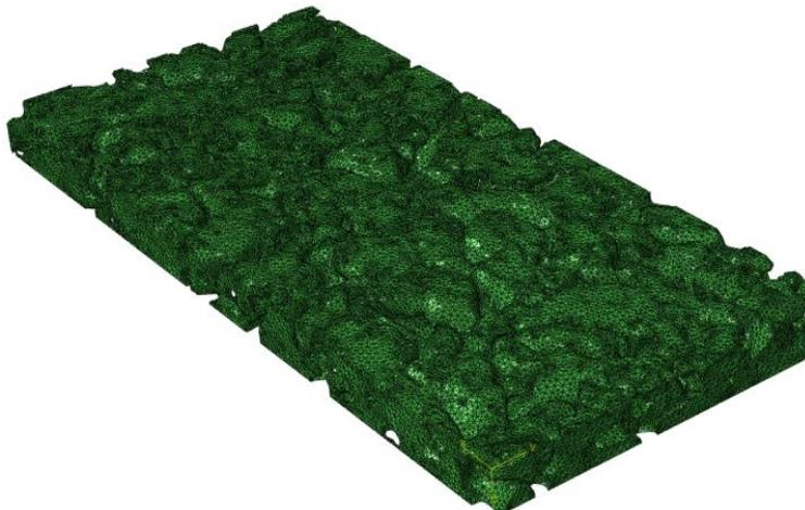
Figure 3.17 3D FE asphalt concrete mesh
