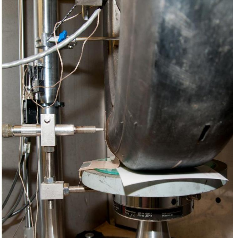
Figure 3.4. Deflection of tire under load
