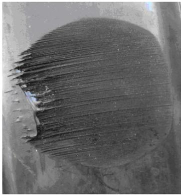
(a) Rubber sample sliced using water jet
