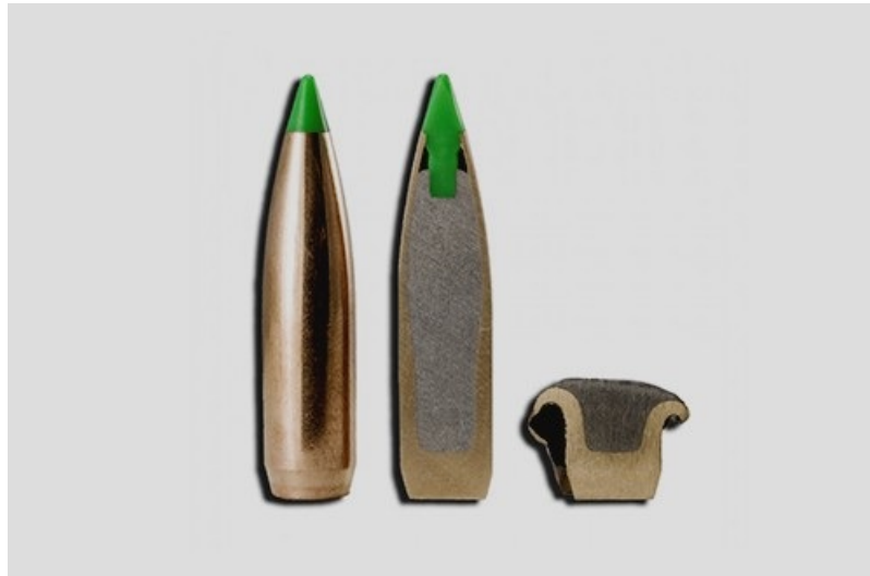
Figure 2.5: BT bullet cross section both before and after firing, taken from [16].
