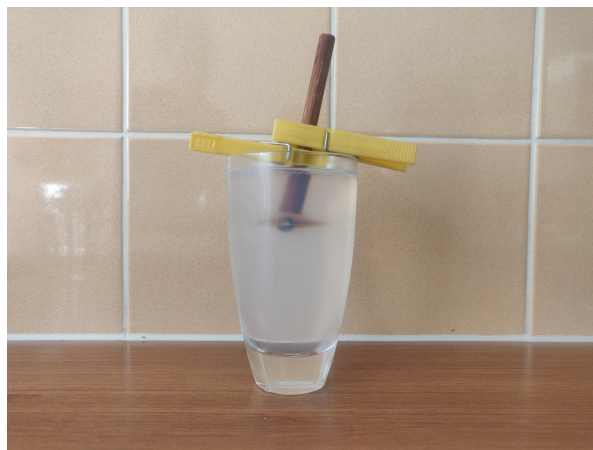
Figure 6.5: The 'phantom' used to test the gripper in, with clothespins to secure the rod in place.
