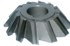
(b) The intended shape for the milling head, taken from [32]
