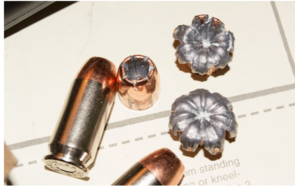
Figure 2.3: HP bullets, before and after firing. Taken from [14].
