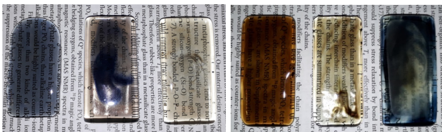
Figure 6: Samples consisting of 12.5% slag melted at different temperatures: 1150°C, 1250°C, and 1350°C, respectively
