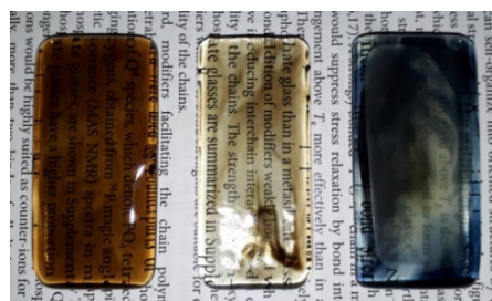
Figure 7: Samples consisting of 15% slag, without the addition of B_2O_3 , with the addition of 10% B_2O_3 and 20% B_2O_3 , respectively
