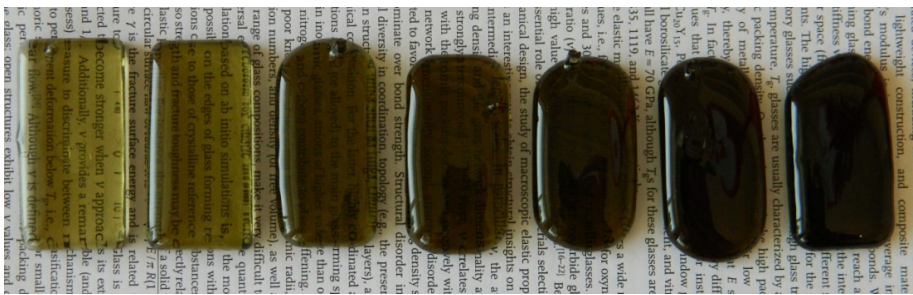
Figure 8: The samples containing fly ash. From the left to the right: 75\text{KPO}_3\text{-}12.5\text{FA-}12.5\text{Al}_2\text{O}_3 , 70\text{KPO}_3\text{-}15\text{FA-}15\text{Al}_2\text{O}_3 , 65\text{KPO}_3\text{-}20\text{FA-}15\text{Al}_2\text{O}_3 , 60\text{KPO}_3\text{-}20\text{FA-}20\text{Al}_2\text{O}_3 , 60\text{KPO}_3\text{-}25\text{FA-}15\text{Al}_2\text{O}_3 , 60\text{KPO}_3\text{-}30\text{FA-}10\text{Al}_2\text{O}_3 , 55\text{KPO}_3\text{-}35\text{FA-}10\text{Al}_2\text{O}_3
