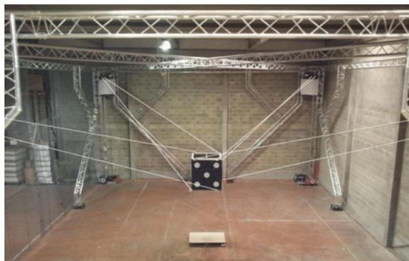
Figure 2.4: The CoGiRo suspended cable robot [17]
