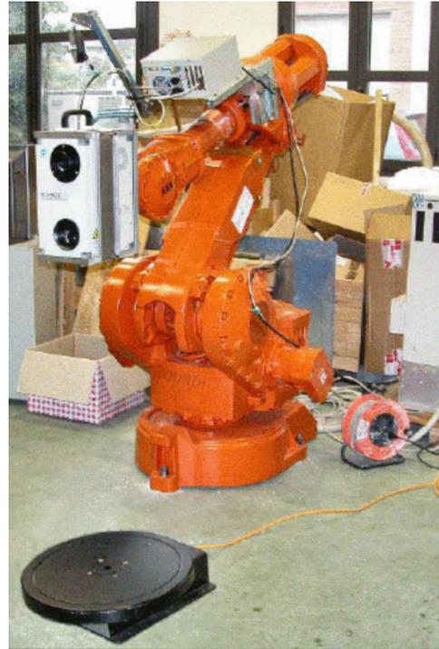
Figure 1.2: An industrial robot arm with rotating platform for the scanning of 3D art. [11].
