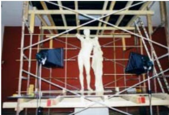
Figure 1.3: Usage of a scaffold around a statue to position a scanner [30].
