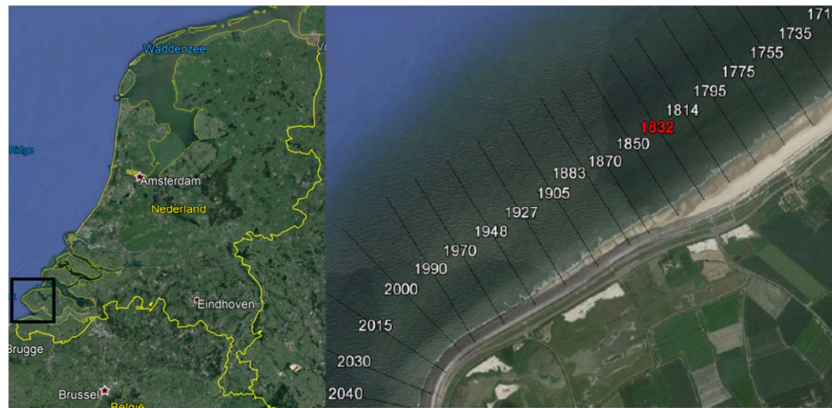
Figure 1. The Netherlands, with the coast of Walcheren indicated (left). The Westkapelle sea defence, with the bathymetrical transects indicated (right). Transect 1832 is shown in red.
