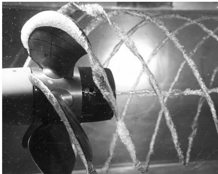
**Figure 1.2:** Cavitation at the tip of the blades and in the trailing vortices in the wake of a propeller in a water tunnel experiment at the David Taylor Model Basin [28].
