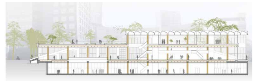
Figure 4.14 Cross-section of CIRCL, demonstrating allocation of functions and void spaces leading natural light to the basement floor (De Architekten Cie., 2017).
