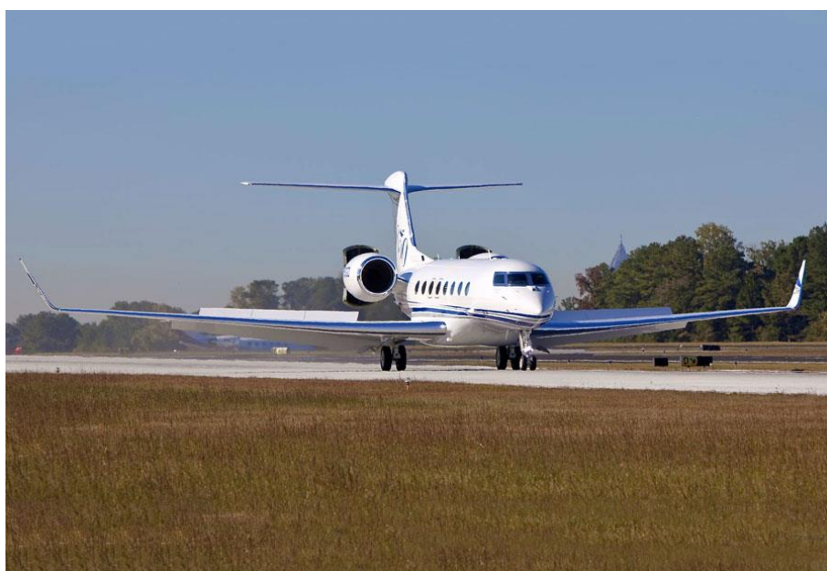
Figure 1.1: Landing Gulfstream G650 with installed Rolls-Royce BR725 engines and deployed thrust reversers (Trautvetter, 2012)
