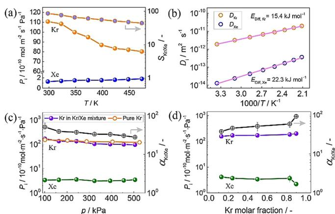
**Figure 3.** a,b) Single component permeation and diffusivity at different temperatures and 1.5 bara. c) Feed pressure-dependent Kr/Xe equimolar mixture separation performance at 298 K. d) Kr/Xe mixture separation performance for different compositions at 298 K and 1 bara. Membrane M2 was used.
