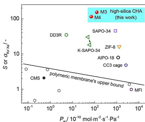
**Figure 4.** Comparison of high-silica CHA zeolite membrane performance in this work with other membranes, including SAPO-34,<sup>[16a-d]</sup> K-SAPO-34,<sup>[16d]</sup> AIPO-18,<sup>[16c]</sup> DD3R, ZIF-8,<sup>[16e]</sup> CC3 cage,<sup>[16f]</sup> carbon molecular sieve (CMS)<sup>[31]</sup> and MFI<sup>[31]</sup> (raw data points given in Table S1). The polymeric membrane's upper bound for Kr/Xe separation is taken from ref. [39].
