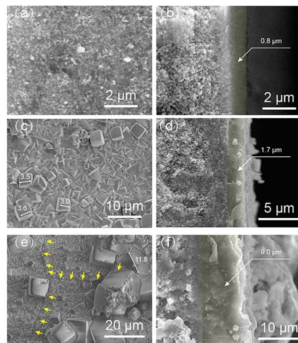
**Figure 1.** SEM image of high-silica CHA zeolite membranes synthesized for 48 h (a,b), 96 h (c,d) and 144 h (e,f). The temperature was fixed at 433 K and the synthesis composition at  $104\text{SiO}_2/1.1\text{Al}_2\text{O}_3/10\text{Na}_2\text{O}/20\text{TMAdaOH}/4410\text{H}_2\text{O}$ . The well-intergrown layer (right, light yellow marker color) and cracks (left, yellow arrows) are highlighted.
