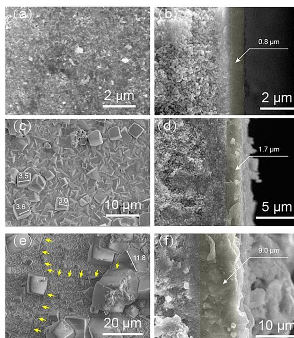
**Figure 1.** SEM image of high-silica CHA zeolite membranes synthesized for 48 h (a,b), 96 h (c,d) and 144 h (e,f). The temperature was fixed at 433 K and the synthesis composition at  $104\text{SiO}_2/1.1\text{Al}_2\text{O}_3/10\text{Na}_2\text{O}/20\text{TMAOH}/4410\text{H}_2\text{O}$ . The well-intergrown layer (right, light yellow marker color) and cracks (left, yellow arrows) are highlighted.
