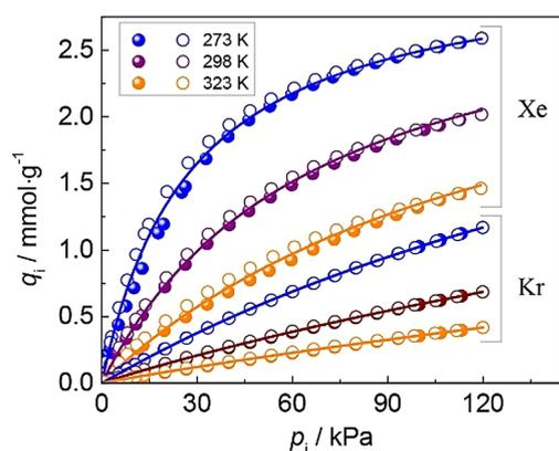
**Figure 2.** Kr and Xe single-component adsorption isotherms of high-silica CHA zeolite (closed symbols: measured adsorption data points; open symbols: measured desorption data points; line: single-site Langmuir isotherm fit).
