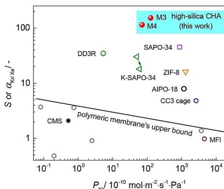
**Figure 4.** Comparison of high-silica CHA zeolite membrane performance in this work with other membranes, including SAPO-34,<sup>[16a–d]</sup> K-SAPO-34,<sup>[16d]</sup> AlPO<sub>4</sub>-18,<sup>[16c]</sup> DD3R, ZIF-8<sup>[16e]</sup> CC3 cage,<sup>[16f]</sup> carbon molecular sieve (CMS)<sup>[31]</sup> and MFI<sup>[31]</sup> (raw data points given in Table S1). The polymeric membrane's upper bound for Kr/Xe separation is taken from ref. [39].
