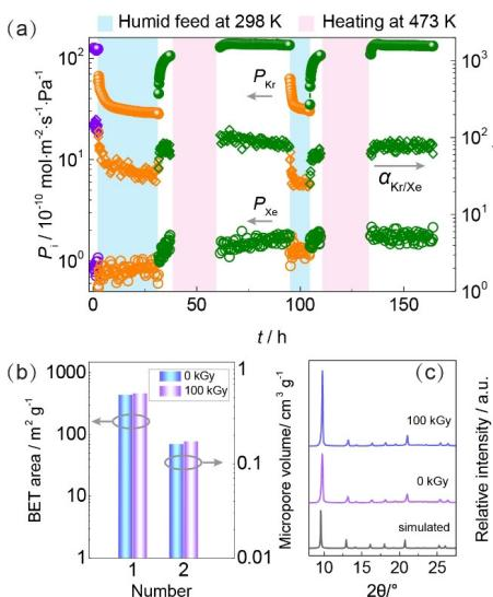
**Figure 5.** a) Hydrothermal stability of high-silica CHA zeolite membrane for dry (purple and green label) and humid (2.3 kPa water vapor, orange label) Kr/Xe mixture separation at 298 K. Membrane M3 was used. b,c) BET area, micropore volume and PXRD of high-silica CHA zeolite before and after  $\gamma$ -irradiation for 30 days and 100 kGy.
