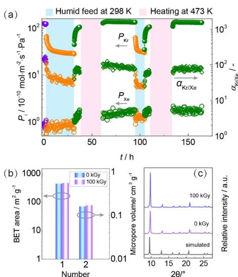
**Figure 5.** a) Hydrothermal stability of high-silica CHA zeolite membrane for dry (purple and green label) and humid (2.3 kPa water vapor, orange label) Kr/Xe mixture separation at 298 K. Membrane M3 was used. b, c) BET area, micropore volume and PXRD of high-silica CHA zeolite before and after  $\gamma$ -irradiation for 30 days and 100 kGy.
