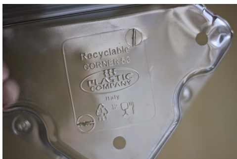
Figure 4.3: a) RIC printed on plastic product [54]. b) Schematic representation of a sink-float set-up [46].
