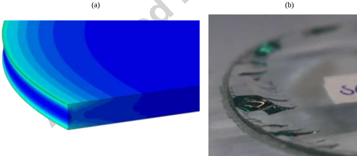
Figure 30: Comparison between results of the finite element numerical modelling and the experimental observation (a) stress field distribution computed by FEM analysis, (b) SG laminated connection failure surface after testing at low temperature
