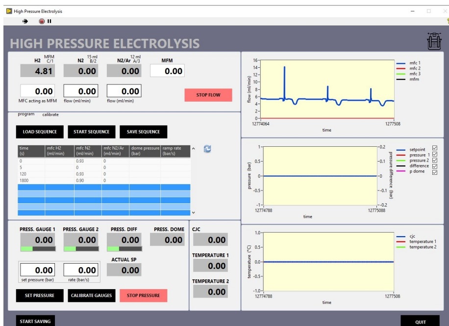
Figure 5.2: An impression of the software that was programmed to control the high-pressure electrolysis system.
