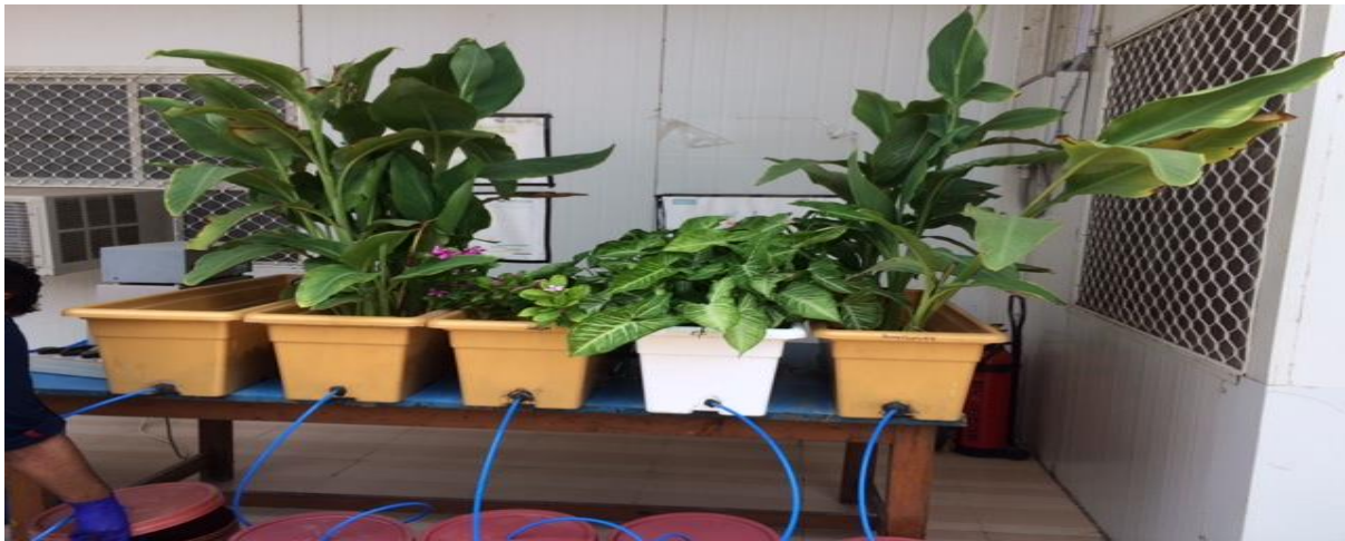
Figure 5 Set-up of constructed wetlands
