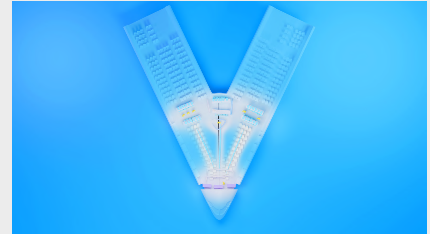
Fig. 87: Flight attendants from workshop 4 suggest one large galley in the centre of the aircraft with a crew chill or resting are potentially in the front. They liked the fact that you could walk through the galley from door to door.
