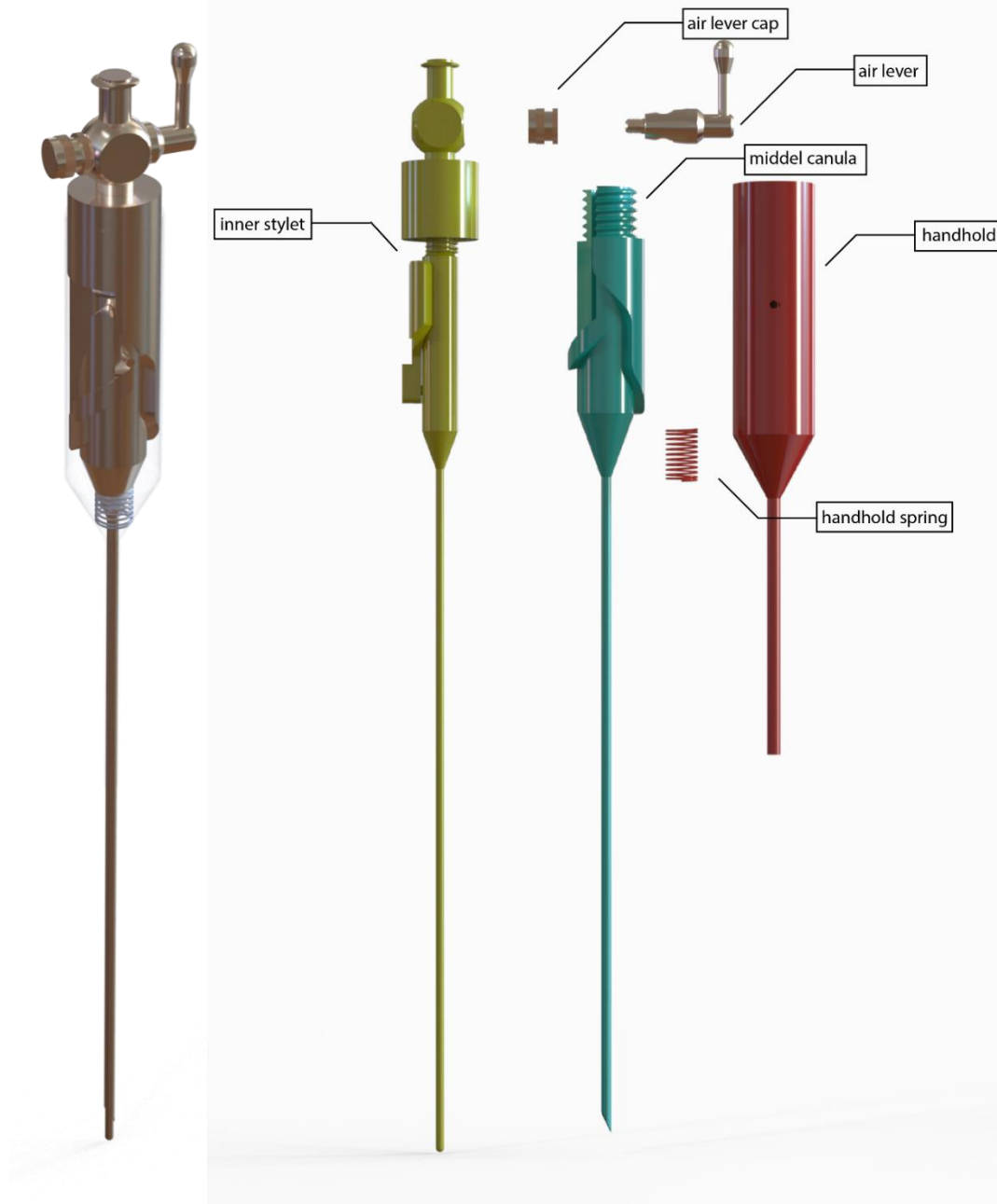
Figure 13: Veress needle based on the clicker concept with transparent handhold and colored components.
