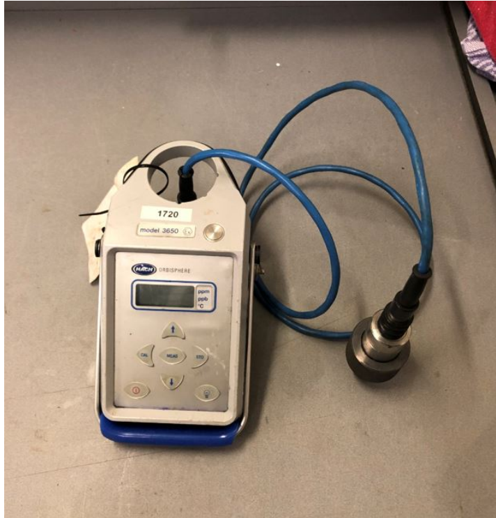
Figure A.3: Orbisphere for measuring oxygen
