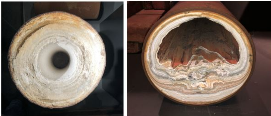
Figure 2.14: Examples of carbonate scale (left) and sulfate scale (right) (Geothermal Museum Larderello, Italy)
