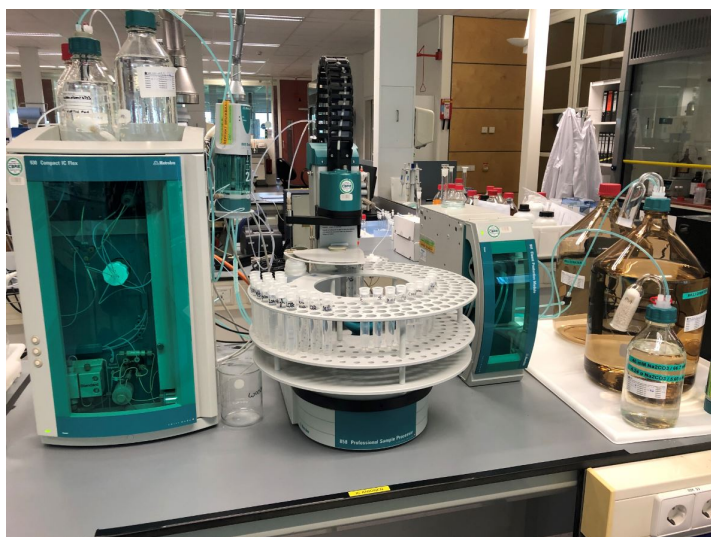
Figure 3.4: Ion Chromatograph for measuring anions
