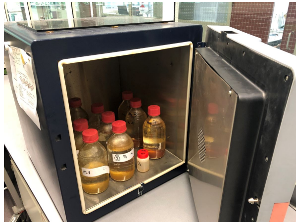
Figure 3.16: Oven for storing samples at high temperatures in the laboratory
