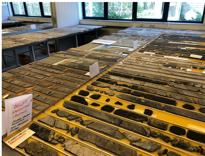
Figure 2.5: Cores of the Delft sandstone member in the core lab of NAM in Assen (02-04-2019)
