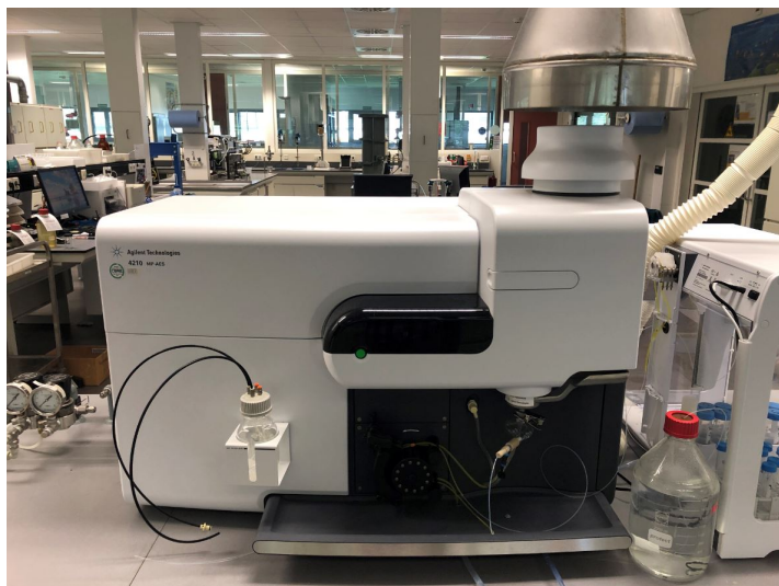
Figure 3.3: MP-AES device for measuring cations
