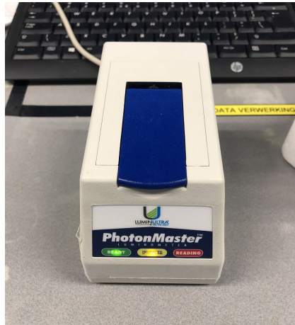
Figure 3.8: Luminometer device to measure ATP. A tube containing sample water and luciferase enzymes is placed into the blue cover
