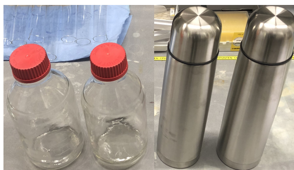
Figure 3.12: Different sample bottles: coated glass bottles (left) and thermos cans (right)
