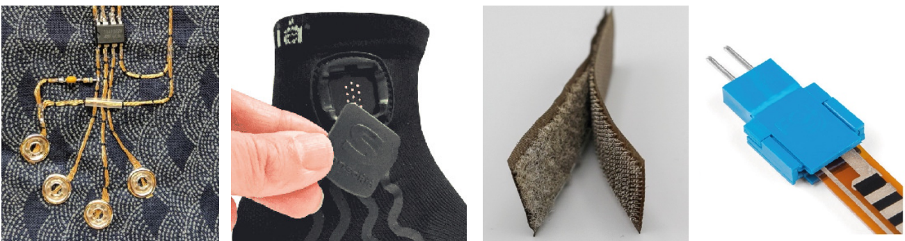
Figure 13: snap fasteners; magnet connector; conductive velcro; pin header (Stanley et al., 2021)
