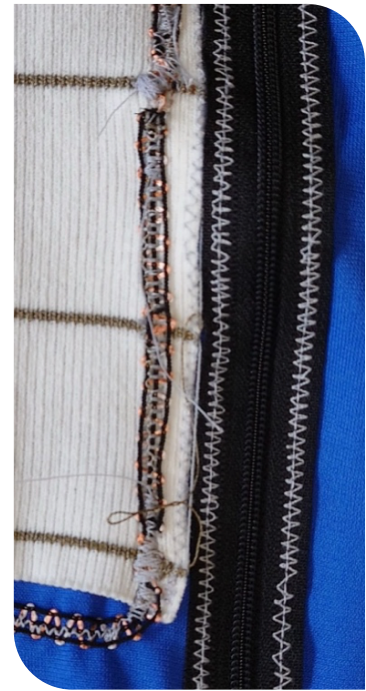
Figure 61: soldered and sewn connections
