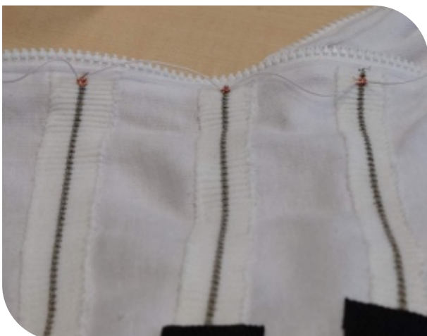
Figure 76: strapping in stripped wires makes up a reliable connection
