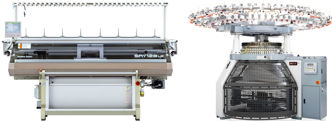
Figure 18: flatbed (Knitting Industry, 2014) vs circular knitting machine (Morton, 2023)
