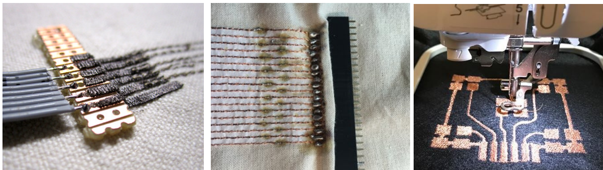
Figure 12: Stitched connection (KOBAKANT, 2009); stitched conductive wires (Staff & Staff, 2021); soldered connection (Instructables, 2019)
