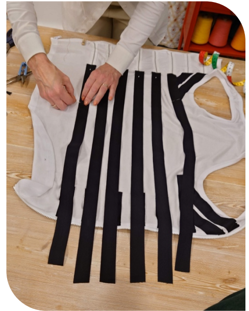
Figure 75: fitting the tensioning straps
