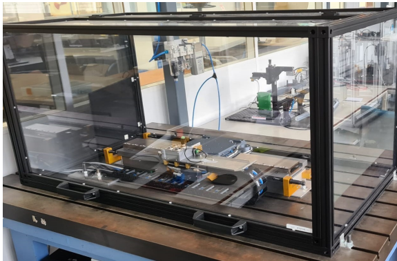
Figure 5.9: The motion stage used for the acceleration sweep measurement. It is a linear air bearing stage with a 500mm stroke range. The high stroke allows for low frequency measurements.
