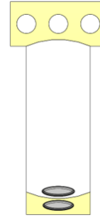
(b) Laser cut buzzer design with soldered connection points. The three holes at the top of the piezo allow for easy tip mass addition.
