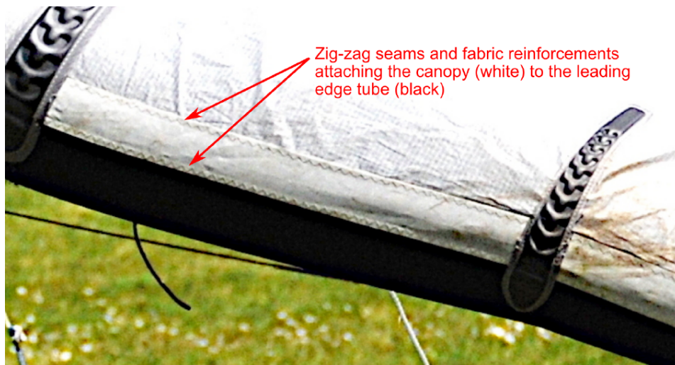
Figure 4.6: Protruding stitched seams near the leading edge of the V3A kite [61].
