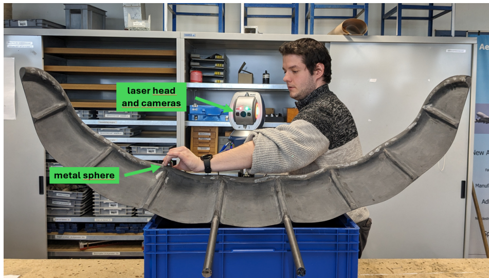
Figure 3.15: FARO laser system and its components.
