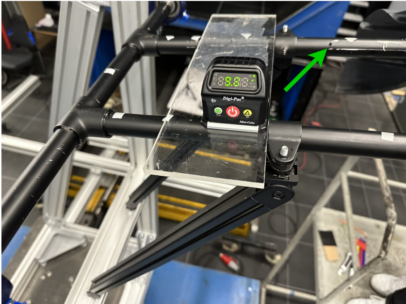
Figure 3.18: Picture of the structure that connects the tubes. The green arrow indicates an adjustment bolt used to fasten the kite to the support structure.
