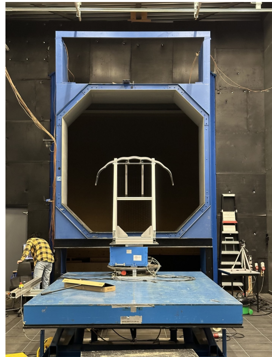
Figure 4.9: Rear view of the experimental setup for the load measurements.
