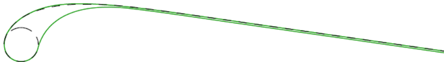
Figure 3.2: Comparison of original airfoil (dashed) and airfoil recreated by Demkowicz (solid) at kite symmetry plane [7].
