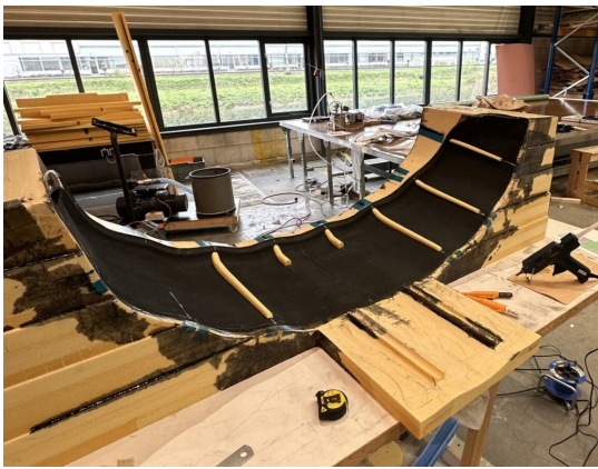
Figure 3.12: V3A kite model being manufactured in its mold.
