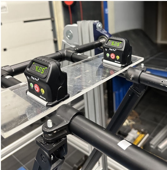
Figure 4.4: Digital inclinometers used to determine the angle of attack of the kite.
