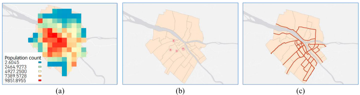
Fig 5: Pontianak criticality analysis model setup: (a) population hotspots from WorldPop as origins of transport demand, (b) healthcare facilities as destinations of transport demand, (c) the main road transport network.
