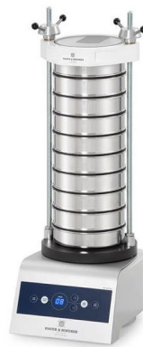
Figure 5.1: Haver EML 200 Premium Sieve shaker with TwinNuts
