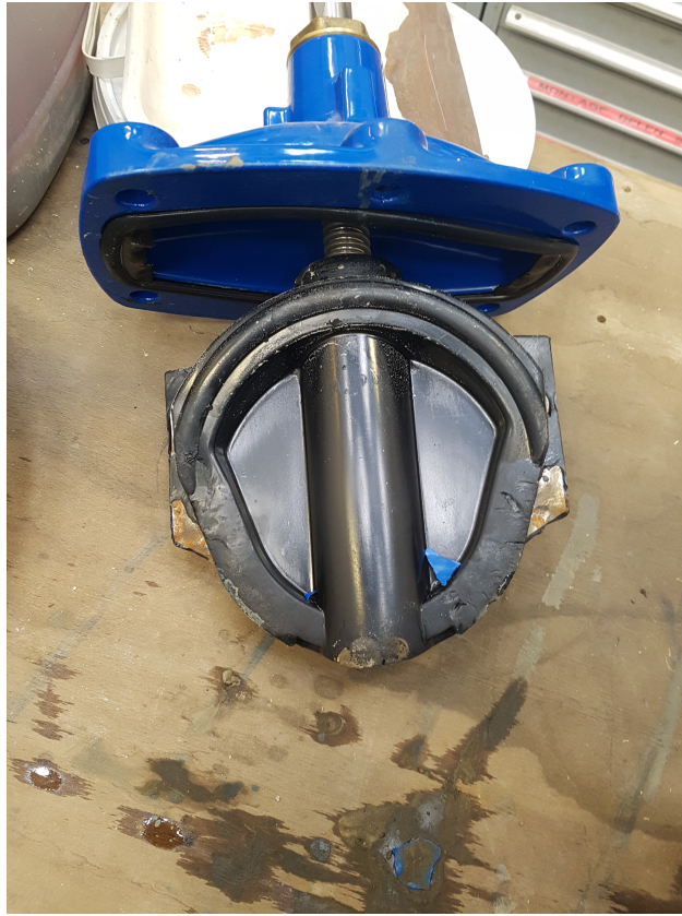
Figure I.6: Gate valve with worn out rubber slide piece
