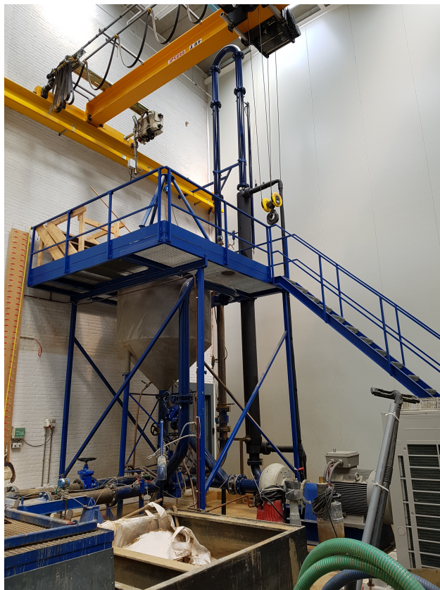
Figure I.3: Overview of the test set up with storage tank and U loop sections
